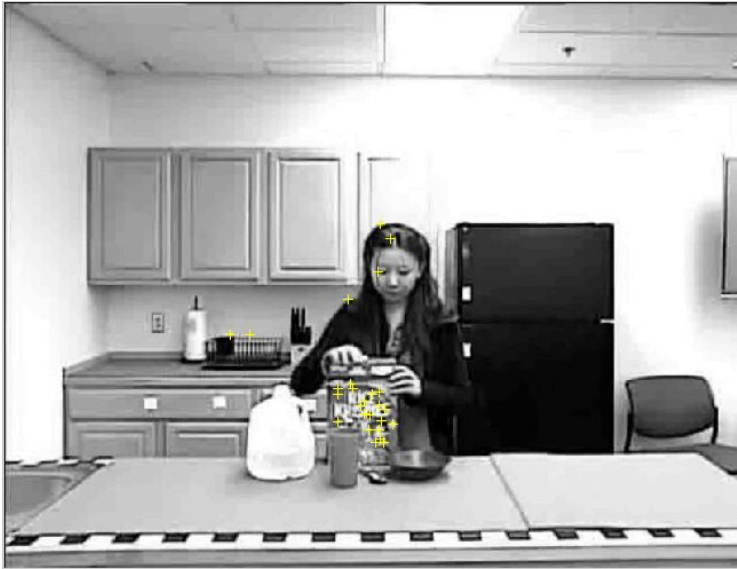
Figure 4.5: Enlarged example of extracted SIFT features from a frame taken during recognition
