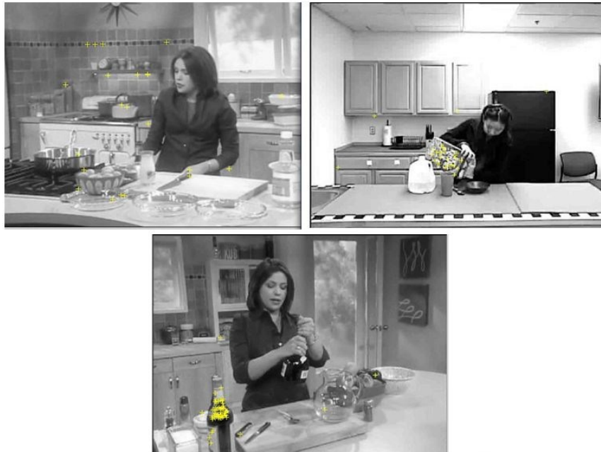
Figure 4.4: Example of extracted SIFT features for frames containing a knife, cereal box, and wine bottle
