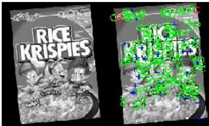
Figure 4.3: Enlarged example of cereal box SIFT model extracted from a training example
