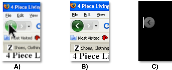
Figure 36 A) The user is pressing on the “Back” button in Firefox (the cursor here is for illustration only and not captured in our data). B) The image captured after the user releases the locator. C) The bounding box around the resulting difference is the correct target.
