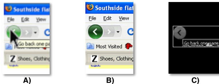
Figure 37 Example of a visual change error in difference imaging: New visual content appears that overlaps or touches target. A) When the user presses the pointer button, a tooltip appears overlaps the target. B) When the pointer button is released, the tooltip disappears. C) When the two images are subtracted from each other the resulting difference region includes both the target and the tooltip, which is incorrect.
