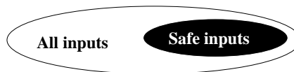
Figure 4.1: An input validation vulnerability occurs when the domain of inputs for a program (white) is a super-set of safe inputs (black).
