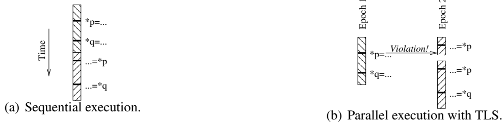
Figure 2: How TLS ensures that all reads and writes occur in the original sequential order.
