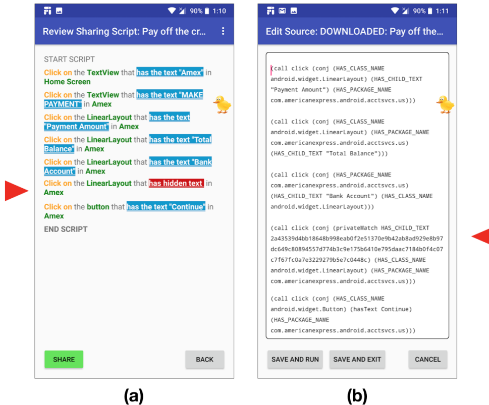
Figure 8.5: The result of processing the script shown in Figure 8.3. The left side shows the review interface for the script author, where the identified personal information is highlighted in red. The right side shows the source of the processed script, where the content of identified personal information is replaced by its hash.
