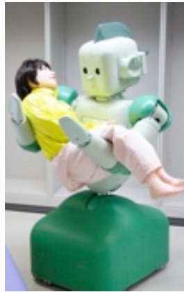
Figure 2. RI-MAN, a robot to lift and carry people. The Institute of Physical and Chemical Research at Nagoya, Japan.
