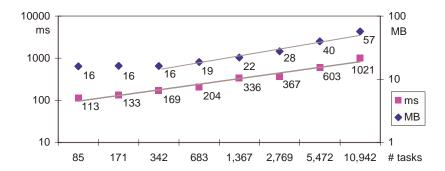
Fig. 9. Latency of task searching and TM memory footprint
