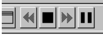
Figure 4.35: The history control buttons are part of the toolbar. The arrow buttons are used to move back and forth in the history and the stop and pause buttons are used to affect timer widgets globally.
