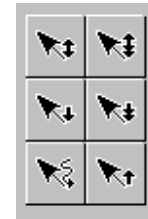
Figure 4.31: The player input icons or “mouse icons.” Each icon represents a kind of mouse event. The double arrows are clicks. The others are down, move/drag, and up event. Double arrows pointing down are double clicking events.
