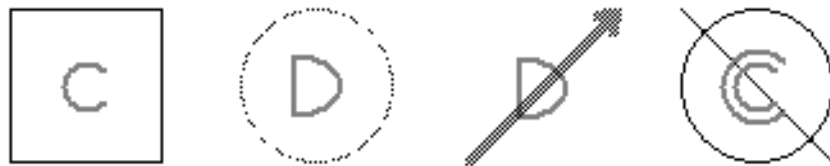
Figure 4.34: Creation and deletion markers. Objects marked with a “C” have just been created. Objects marked with a “D” are deleted (which is sometimes visible on the deleted object’s ghost as well). When two or more markers would overlap, the markers grow so they nest.
