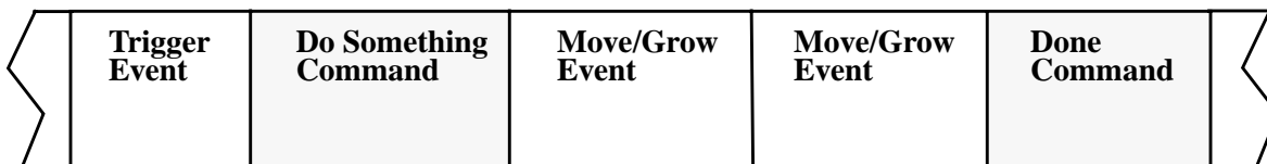
Figure 5.9: After the first demonstration, Gamut's undo history list contains the events that correspond to the developer's example. The actual editing events are enclosed between the Do Something and Done commands. All examples end with the Done command.
