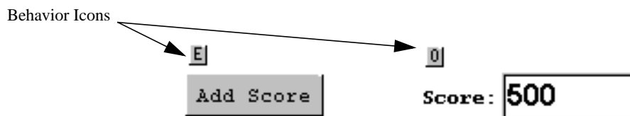
Figure 8.3: Here a button and number box are marked with “behavior icons” to show that they have had a behavior defined for them. The “E” marker indicates that the button’s event is used for a behavior and the “O” marker shows that the number widget will be affected.
