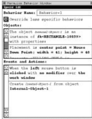
Figure 2.5: Marquise’s dialog for editing code. The items in bold text could be selected to provide dialogs and menus that would let the developer choose different code fragments. [76]
