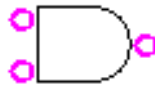
Figure 4.7: This And gate uses little circles as guide objects to show where wires may be attached.
