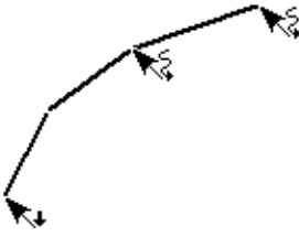
Figure 4.33a: Demonstrating a free hand line behavior requires the developer to have an intermediate moving point.
