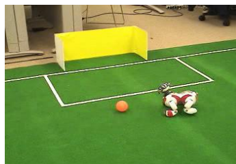
Case (2b): The robot looks to the location of the kick success hypothesis for the ball but doesn't find it.
