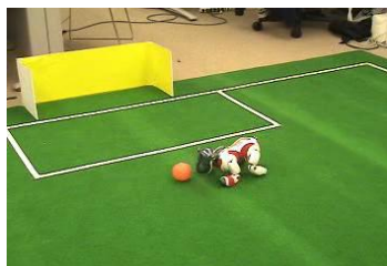
Case (2a): In a different kick, the open-loop grab and kick fails.
