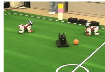
Case (3c): All of the kick hypotheses expire and the robot tracks the teammate's reported hypothesis (the ball is hidden from the first robot's view.)
