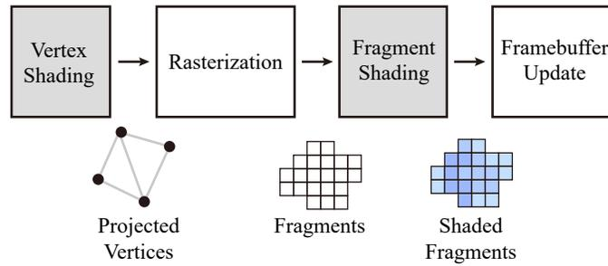
Figure 2.8: The GPU graphics pipeline architecture. Pipeline stages are shown in square boxes. Boxes in gray background represent programmable pipeline stages, and boxes in white background represent fixed-function stages.
