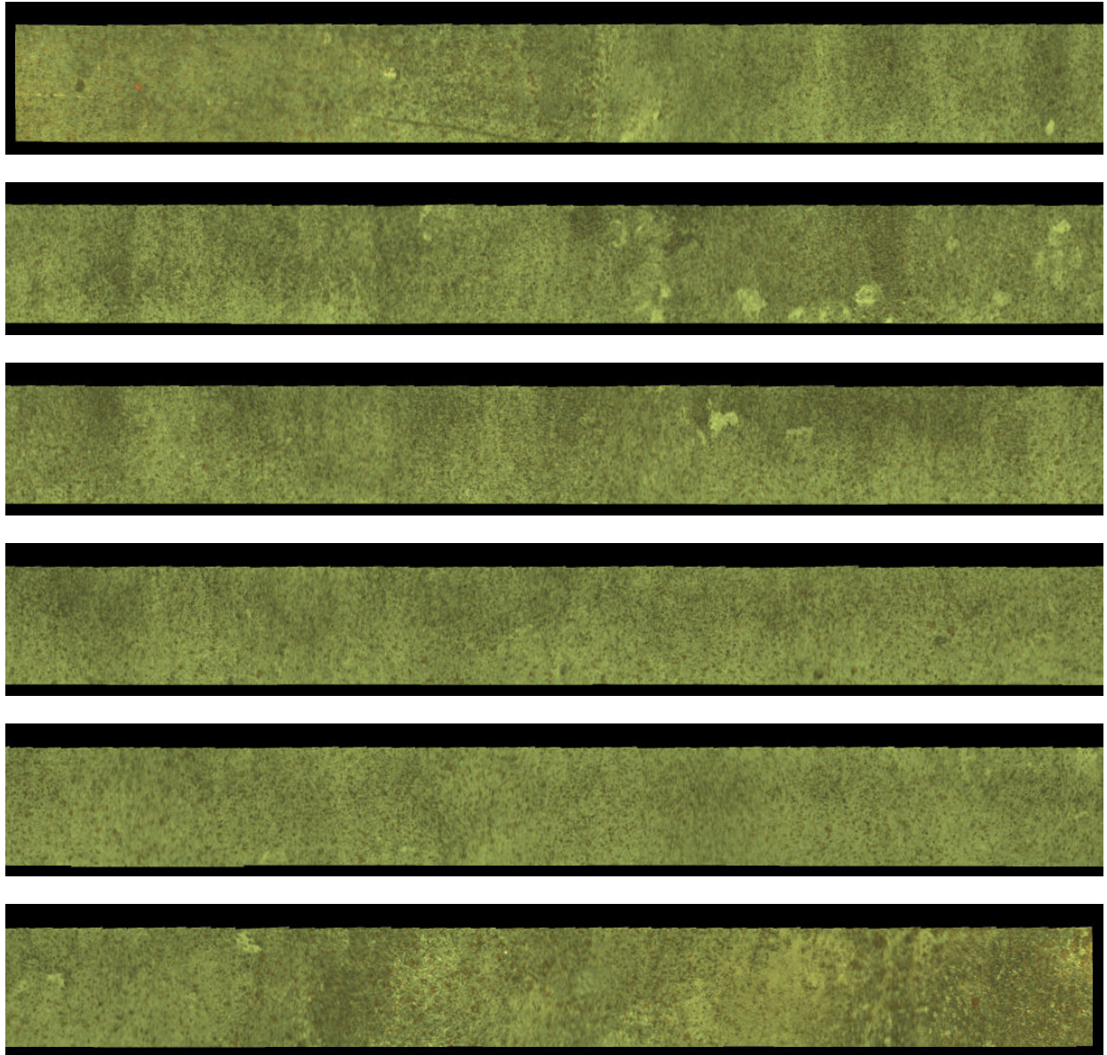
Figure 17: The tiled stitched image for the pipe 2 (4 meters long 406.4mm (16") diameter) dataset (forward) obtained using the sparse algorithm. The images are stitched on the surface of the pipe, where a u, v coordinate in the stitched image corresponds to an h, \rho = r\phi coordinate on the surface of the pipe.
