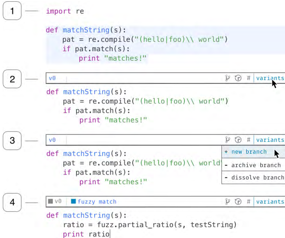
Figure 7.3 Variolite’s “variant box” interaction. In (1) the user highlights a region of code with their cursor that they are interested in experimenting with. In a right-click menu option they select “wrap in variant”, and in (2) a variant box appears above their selected code. The user now has the option of adding variants to this code, which they do by clicking on the variant box header and selecting “new branch” (3). In (4) the user has created a new variant for their code. They can switch between their variants by clicking the variant’s title.
