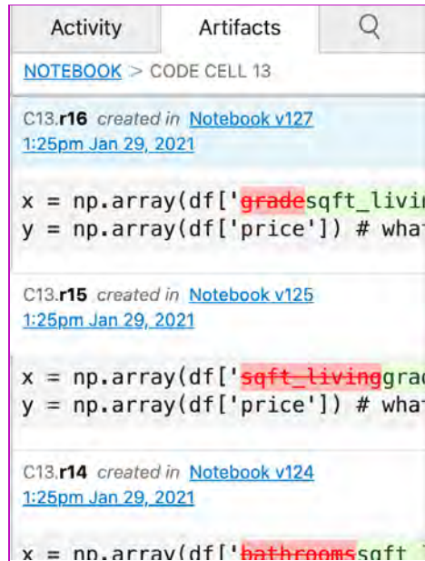
Figure 14.7 Cell naming conventions in Artifact Detail view. Here C13.r16 means the 16th version (r for “revision”) of the 13th code cell that the user created. In practice this was confusing to users.
