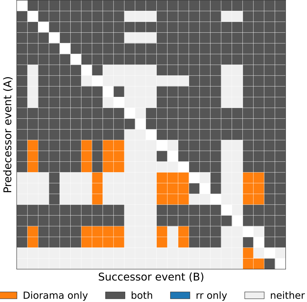
Figure 5.5: Categorical heatmap of happens-before pairs explored by each tool. Orange cells indicate pairs explored only by DIORAMA; dark grey cells indicate pairs explored by both tools; light grey cells indicate pairs explored by neither tool. No pairs are explored exclusively by rr (blue). DIORAMA explores a strict superset of the orderings that rr reaches.
