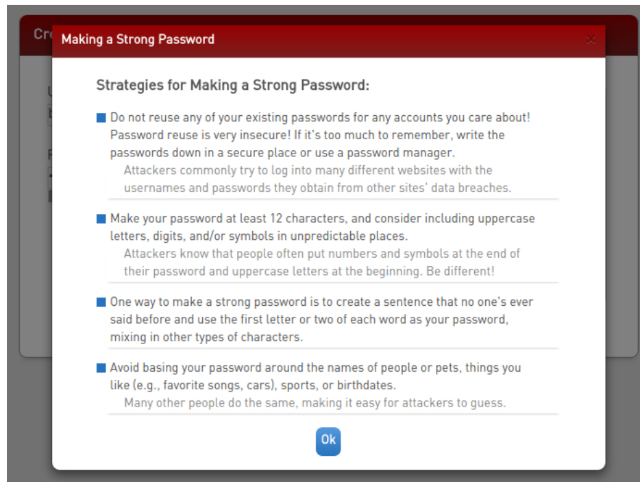
Figure 7.5: The meter’s generic-advice modal window, which warns against password reuse and provides guidance about strategies for creating strong passwords, as well as highlighting predictable decisions to avoid.
