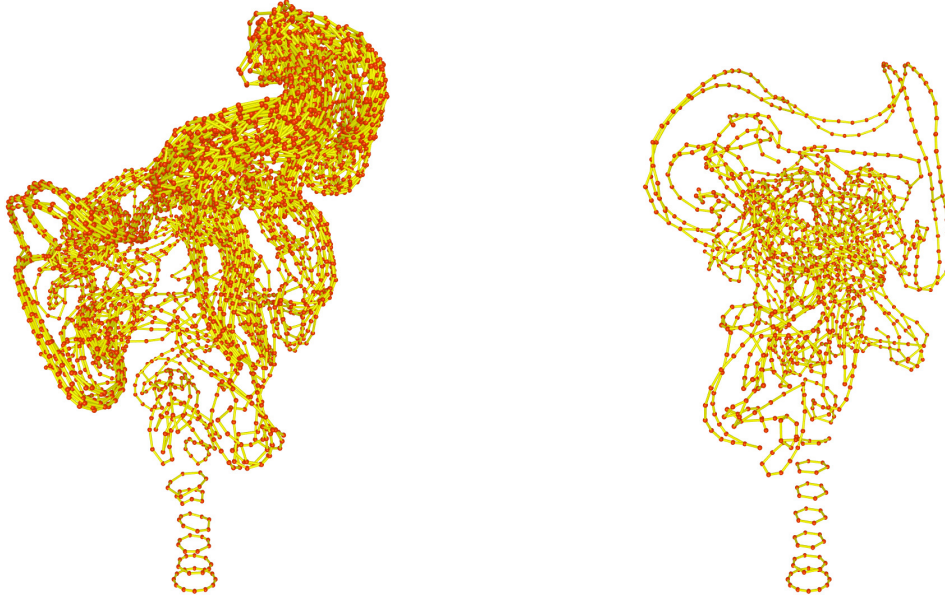
Figure 3: Without reconnection, thick bundles of vortex filaments form ( left ). With reconnection, the simulation contains \frac{1}{3} the number of filaments, though a small amount of viscosity is introduced ( right ).
