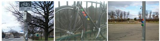
Figure 3.4. Cyclist sensor placements: exhaust and dust probes at a bike lane; all sensor probes attached to bike; exhaust, dust and chemical probes in public park.
