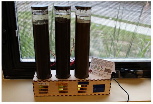
Figure 6.1. Bio-electronic soil sensing device deployed at an environmental outreach community center.
