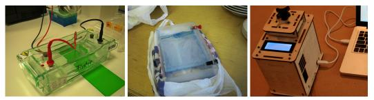
Figure 7.3. Gel electrophoresis box in a professional lab (left) and assembled from scratch at London Hackspace (center); OpenPCR kit for replicating DNA.
