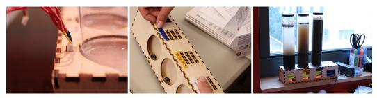
Figure 6.6. Designing a bio-electronic system: column plugged into casing; labeling the column slots; testing the system.
