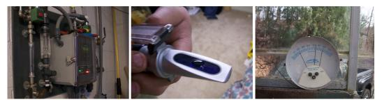
Figure 5.2. Technologies used by participants: ORP probe, routinely used to monitor ozone levels in aquariums, refractometer, occasionally used to check honey before harvesting; thermometer, checked daily.
