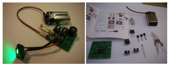
Figure 4.4. Air quality balloon kit: sensing board fully assembled and board, instruction booklet and all components.
