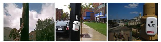
Figure 3.9. Photographs of participant sensor placements: participant's daughter attaching VOC sensor to street pole; and exhaust sensor outside a children's hospital placed by activist; dust sensor attached to bridge by bicyclist.
