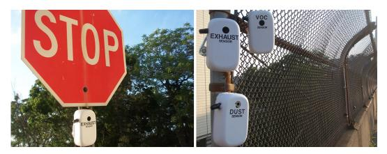
Figure 3.6. Functional place-based sensors: exhaust sensor attached to stop sign; dust, exhaust and VOC sensors attached to bridge.
