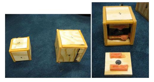
Figure 2.5: The interior and exterior of a force sensing cube. The construction is similar to the spoon; sensors are placed between plates at junctures.
