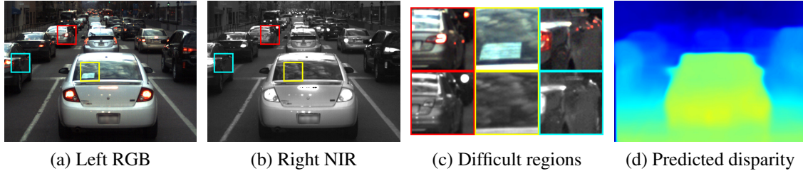
Figure 5.2: A challenging case for RGB-NIR stereo matching and our result. Cyan box: The light source is visible in RGB but not in NIR. Yellow box: The transmittance and reflectance of the windshield are different in RGB and NIR. Red box (brightened): Some light sources reflected by the specular car surface are only visible in RGB. Our approach uses a deep learning based simultaneous disparity prediction and spectral translation technique with material-aware confidence assessment to perform this challenging task.
