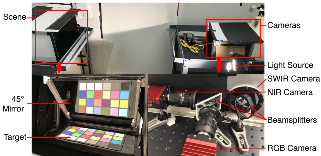
Figure 2.3: Image Acquisition System. RGB, NIR, and SWIR cameras are co-located using beamsplitters. The target is imaged through a 45° mirror.
