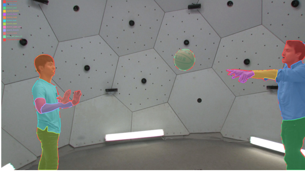
Figure 4.3: Canonical-frame semantic ownership. SAM2 segments foreground objects such as the ball, while SAPIENs separates human body parts. These labels are computed once on the canonical frame and then reused throughout the stream to define which Gaussians should move together.
