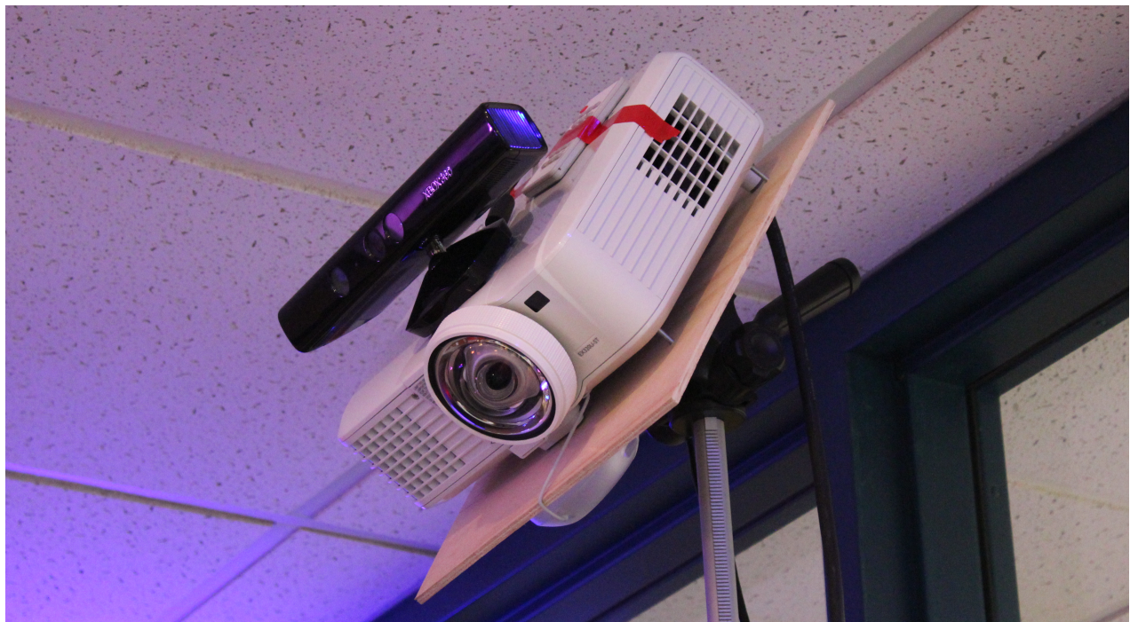
Figure 4.3. A short throw projector with mounted Kinect.
