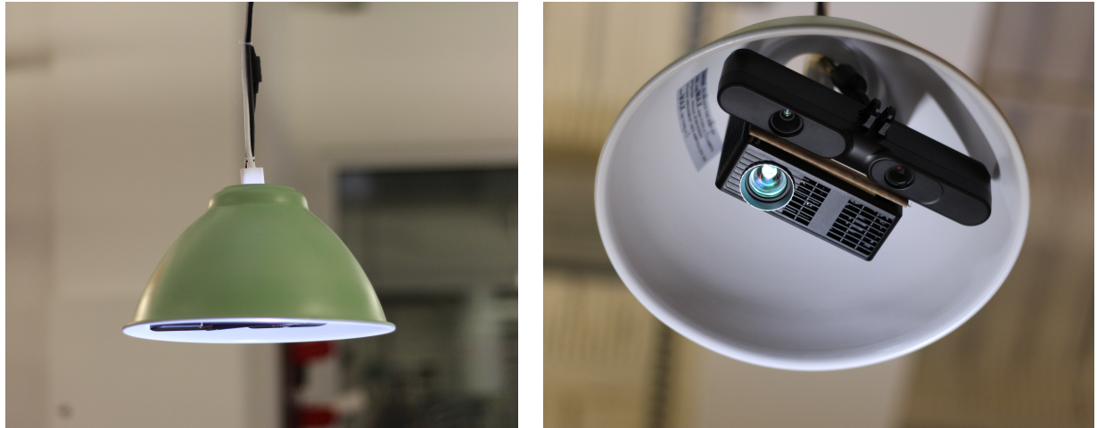
Figure 5.9. Our proof of concept projector-camera system fitted into a lampshade.
