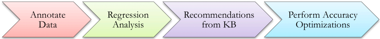
Figure 5.2: A visualized representation of the sub-steps used in identifying the significant degrading factors in speech recognition results, as in Step 3 of the ChAOTIC process framework.
