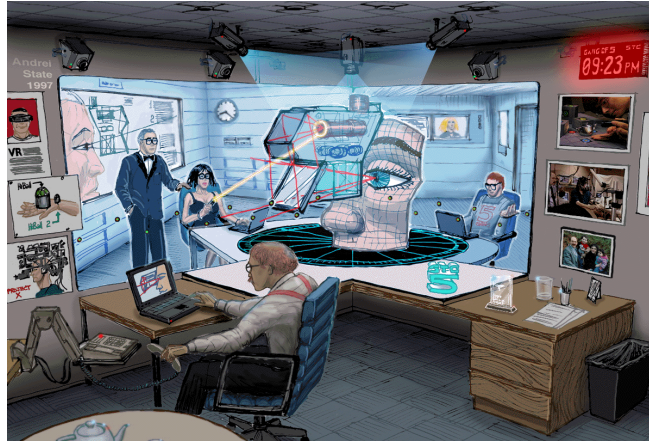
Figure 2.8. Conceptual sketch of the Office of the Future, a spatially immersive workspace using large projection instead of standard desktop monitors.
