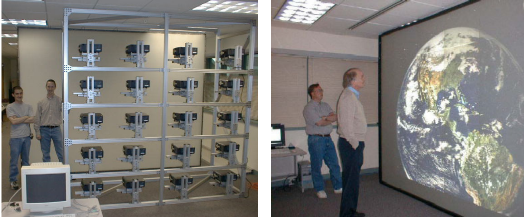
Figure 2.1. The NCSA Display Wall-In-A-Box is a 20 projector array carefully stitched together to form a single large high-resolution display.
