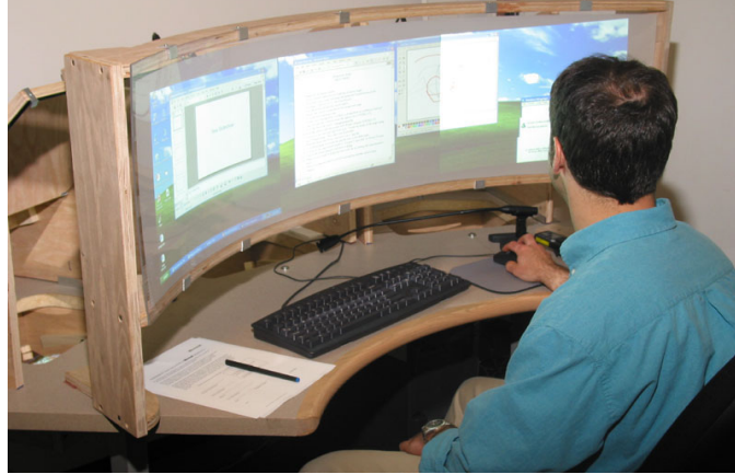
Figure 2.10. The Dsharp widescreen display has facilitated studies exploring the effects of wide fields of view in productivity as well as spatial tasks.
