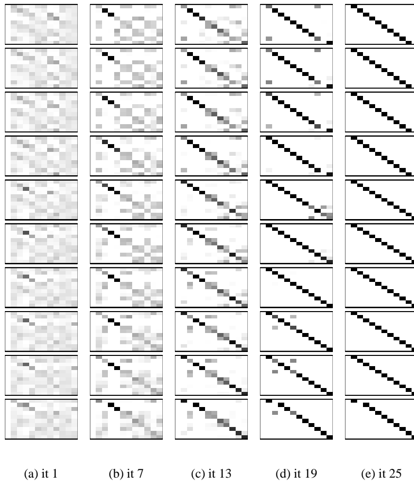
Figure 8.5: Marginal probabilities computed in the E-step. Occlusion shows up as breaks in the “perfect” correspondence matrix (an identity matrix). In this example, the first four images are missing a measurement on the last feature, whereas the last image does not have an observation on feature 2.
