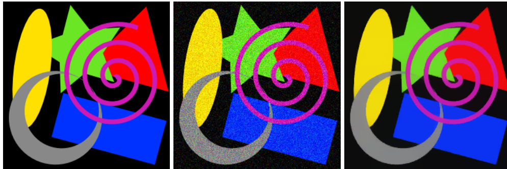
Figure 6.6: Left: original image. Middle: image corrupted with Gaussian noise. Right: image recovered with total variation using proximal Dykstra and ASPN.
