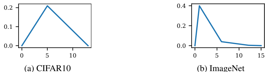
Figure 4.6: Cyclic learning rates used for FGSM adversarial training on CIFAR10 and ImageNet over epochs. The ImageNet cyclic schedule is decayed further by a factor of 10 in the second and third phases.
