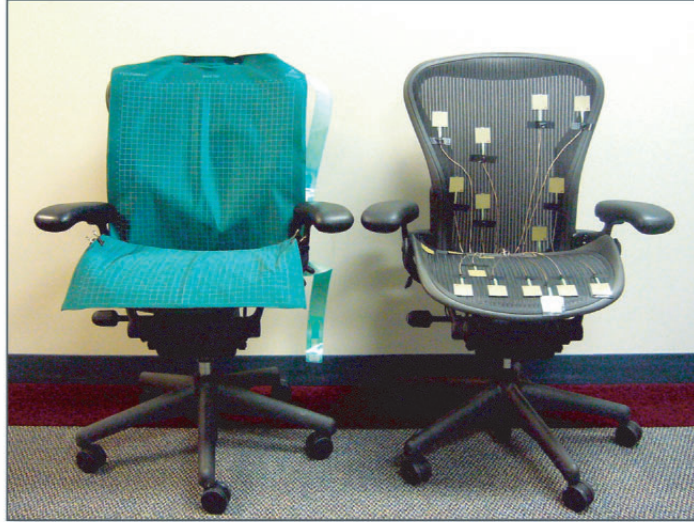
Figure 7.4: On the left is the commercially-available high-resolution Tekscan ConforMat sensor (with 2048 sensors) installed on a Herman Miller Aeron Chair. On the right is our deployed system (with 19 sensors) installed on the same chair.
