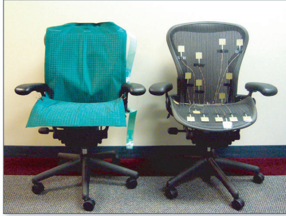
Figure 1.5: Expensive high fidelity sensor (4032 point sensors). We achieve comparable classification accuracy using only 20 flat and point sensors.
