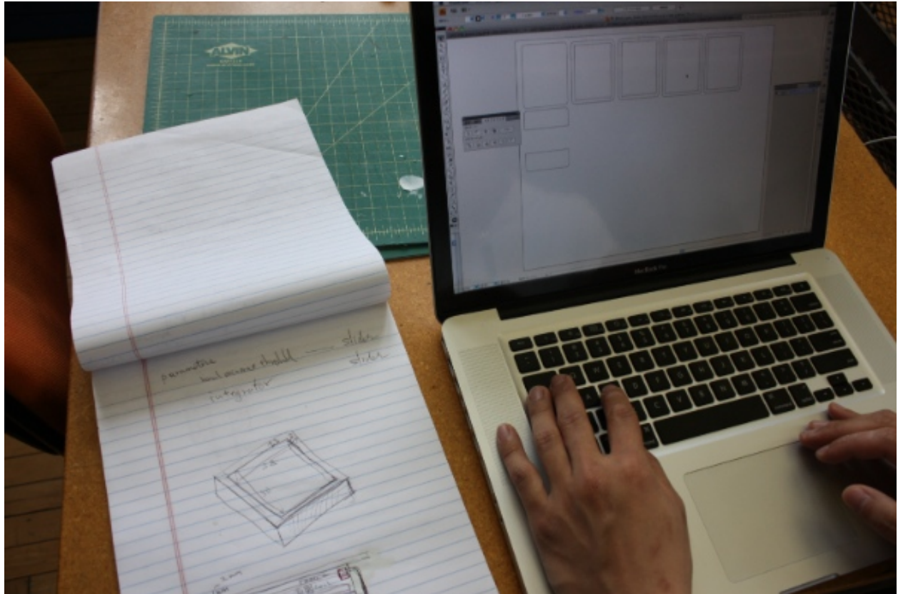
Figure 4: A common step of designing for laser cutters: translating a hand-made sketch to a computer modeling tool. The sketch includes a perspective drawing of the desired result, and 2D diagrams of individual parts with key dimensions indicated.
