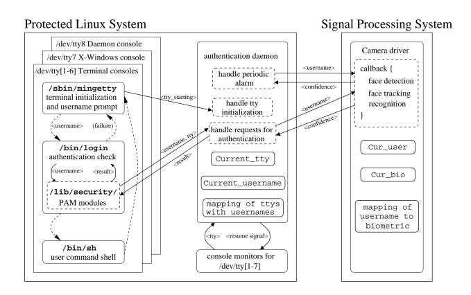
Figure 2: Implementation of Continuous Video Enhanced Authentication System
