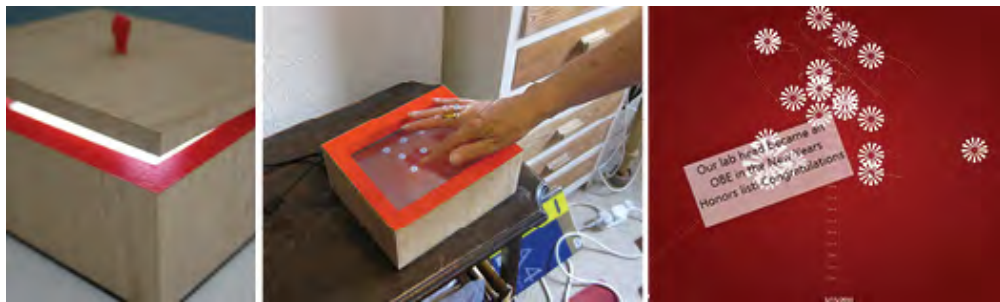
Figure 4. From left to right: The removable lid; Mom2 presses a icon to open a Tweet; UI design for an opened Tweet.
