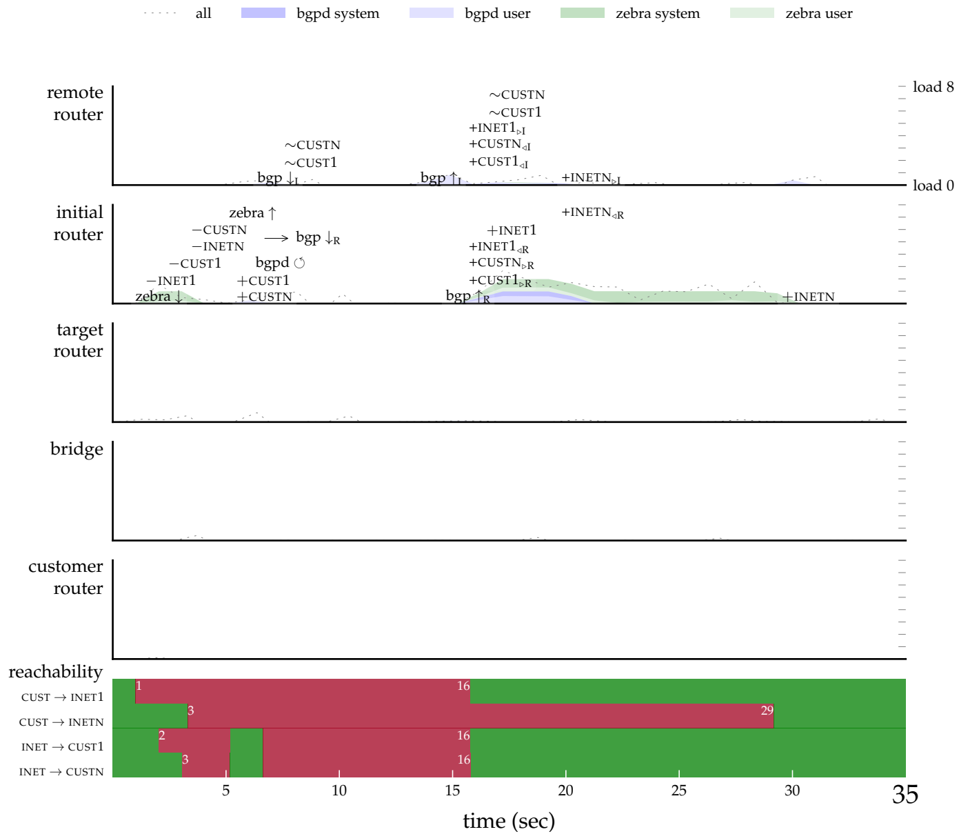
Figure A.4: Full system chart for router restart with a single static customer, on High Spec hardware. This chart illustrates the trial with the shortest overall outage time.
