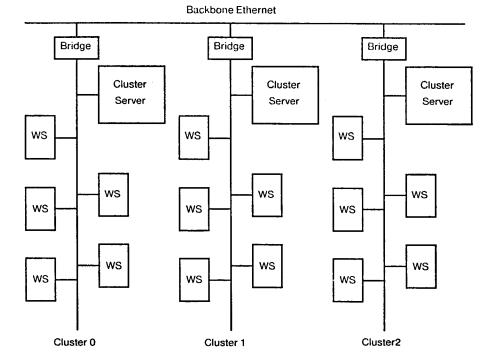
Each WS is a Virtue workstation. We expect a cluster to contain between 50 and 100 workstations. The final system that spans the CMU campus will have a total of about 100 clusters
