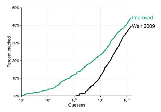
Figure 7.6: Experiment 9A — Evaluating two 4class8 models. The *Weir 2009* model used settings akin to Weir's original approach [146] when learning a PCFG, while the *Improved* model incorporates improvements from this thesis: quantized string frequencies, hybrid structures, and unseen terminal generation.
