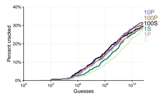
Figure 6.10: Experiment 6 — Guessing curves for six conditions where we manipulated the weight of password samples from the target policy (3class12). We find that weighting has little effect on guessing performance in this case, though weighting is generally better than building models with only public data (the 0 curve). See the text for an explanation of the weighting schemes we used.
