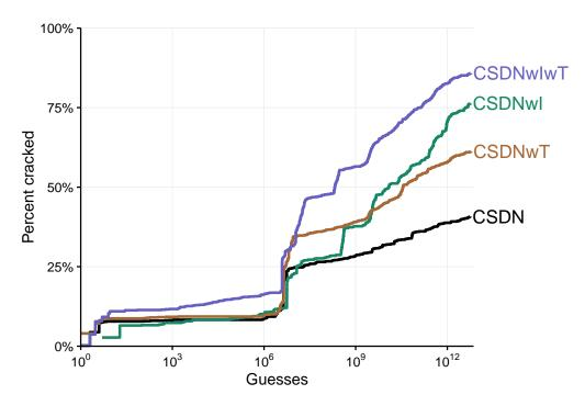
Figure 7.3: Guessing curves for CSDN passwords across all four experiments from Figure 7.2 (wI = with *Improved* model, wT = with additional training data)
