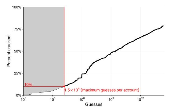
Figure 6.4: Experiment 1 — The area above the guessing curve and up to a maximum number of 15,347 guesses. The total shaded area approximates the  $\alpha$ -guesswork needed to crack 10% of passwords. Note that the x-axis is in log-scale, so the area as shown is not the *true* area of the region.
