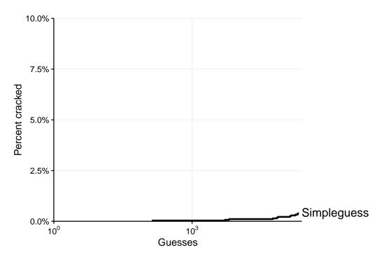
Figure 3.2: Guessing curve for a 3class12 policy using the *Simpleguess* guessing model. 2,774 passwords were collected from Mechanical Turk for testing. All 3class12 passwords from the RockYou dataset were used for training. Note the y-axis limit is at 10% cracked. The guess cutoff, i.e., the total number of guesses made by the Simpleguess algorithm, is 200,809.
