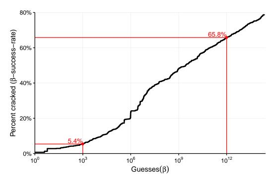
Figure 6.2: Experiment 1 — Guessing curve for the basic8 policy, annotated for  $\beta=10^3$  and  $\beta=10^{12}$  guesses. The percentages above each point show the estimated  $\beta$ -successrate for the corresponding number of guesses, based on the test sample.
