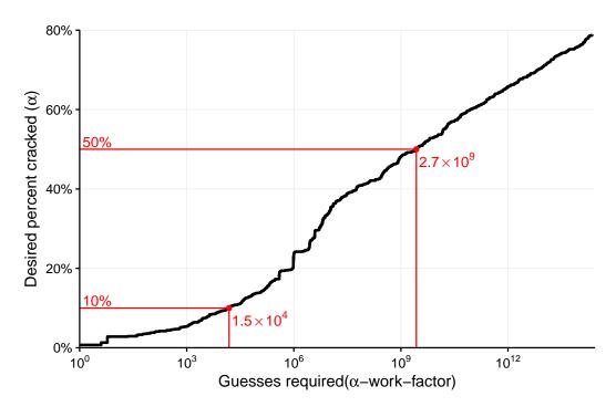
Figure 6.3: Experiment 1 — Guessing curve for the basic8 policy, annotated for  $\alpha = 10\%$  and  $\alpha = 50\%$  as the desired percentage cracked. The numbers beside each point show the estimated  $\alpha$ -work-factor, or the required number of guesses, based on the test sample.
