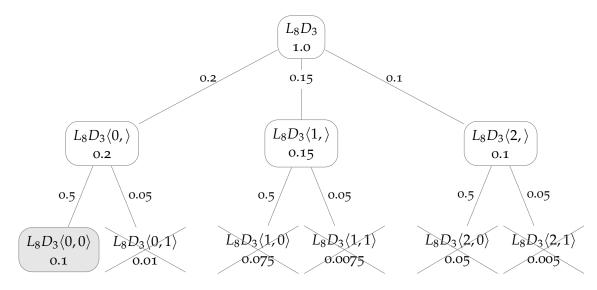
Figure 4.8: SST after applying Algorithm P with a probability cutoff of o.o8. Visited nodes are outlined, nodes whose patterns were recorded are shaded, and nodes whose patterns were rejected (below the cutoff) are crossed out. Only one pattern was recorded, but all nodes were visited because no internal node had a probability less than the cutoff.
