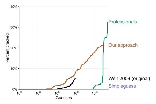
Figure 3.7: Experiment 12 — Guessing curves for the 3class12 policy generated using the Simpleguess algorithm, Weir's original 2009 PCFG implementation [146], our improvements to Weir's PCFG approach, and professional crackers. Our approach represents 16,903,290,362,610 guesses and cracks 21.4% of passwords. The configuration for this experiment is provided on page 233.
