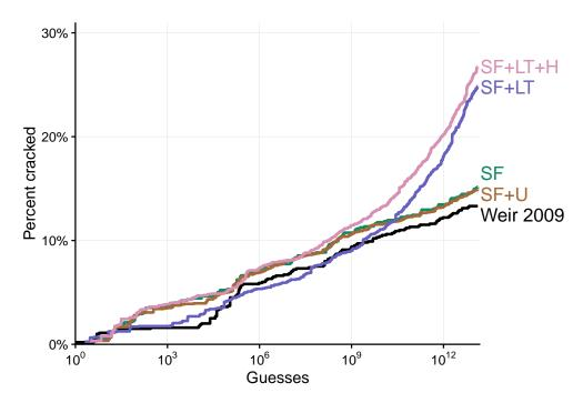
Figure 7.8: Experiment 4 — Evaluating the basic16 policy using various configurations of the guess-calculator framework. The Weir 2009 model used settings akin to Weir's original approach [146]. The other models enable various improvements: SF = quantized string frequencies, U = unseen terminal generation, LT = linguistic tokenization, and H = hybrid structures. The improvements are described in Chapter 5.
