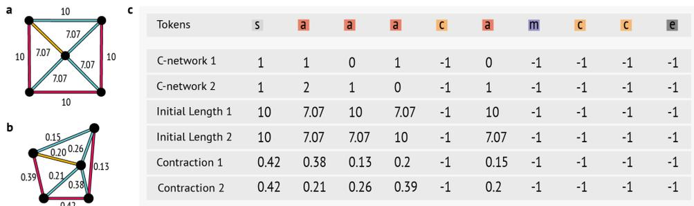
FIGURE 6.7: **2D Truss Grammar parameters.** **a.** A truss before transformation initialized with C-network indices and initial edge lengths. **b.** A truss after transformation with each C-network contracting, with numbers showing the contraction ratio of each edge. **c.** Top: The topology tokens representing the truss in **a**, **b**. Bottom: Pairs of C-network indices, initial edge lengths, contraction ratios corresponding to each token.
