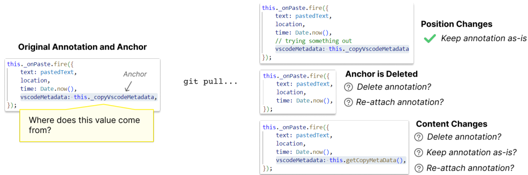
FIGURE 5.1: An example scenario in which an annotation's anchor is updated in multiple ways after a git pull . In the case only the position changes, the annotation content should stay as-is and the anchor will update to represent the new start and end positions. If the anchor is deleted, it is unclear whether to delete the annotation or to re-attach the annotation at a different, semantically similar point. Likewise, if the content within the anchor's bound changes ( this._copyVscodeMetadata to this._copyVscodeMetadata , in the figure), under different circumstances it may make sense to delete the annotation, keep the annotation on the new anchor content, or re-attach the annotation elsewhere.
