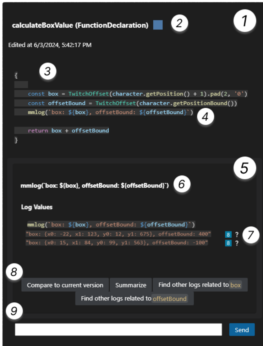
FIGURE 8.3: How an expanded code version appears in MMAI. (1) is similar to Meta-Manager (see Figure 7.2), in that information about the edit is shown including when it occurred and what the code looked like at that point in time, along with any additional meta-information (with this version containing no additional meta-information). (5) shows the optional, supplementary information when mmlog is used, including the log statement (6) (in case multiple mmlog statements exist in one version), most recent log statement and values along with aggregate counts and a button to ask about that value (7), and computed queries that can be sent to the LLM, given the mmlog statement and value (8), along with the option for the developer to write their own query (9).
