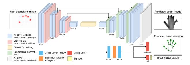
Figure 5.6: TouchPose CNN Architecture. It is a multitask learning framework that takes in a capacitive image as input and predicts the depth image, 3D hand pose, and touch classification for it.
