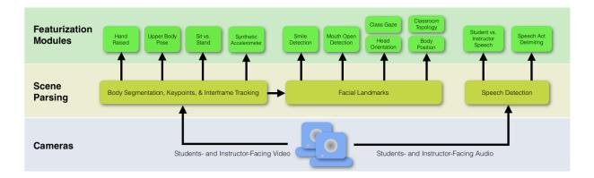
Figure 3.2: Video and audio from classroom cameras first flows into a scene parsing layer which captures the user's pose, before being featurized by a series of specialized modules.
