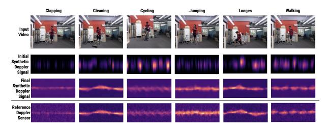
Figure 7.2: Top row shows a user performing different activities. Below each activity is the initial and final synthetic Doppler signal. The bottom row shows the corresponding signal captured by an actual Doppler radar sensor (positioned next to the camera that filmed the user). Note the synthetic pipeline produces comparable signal.
