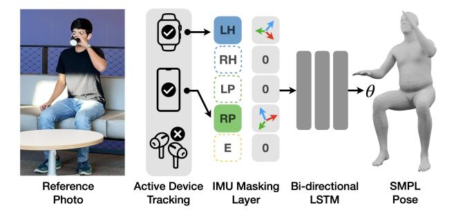
Figure 8.4: Overview of IMUPoser's real-time system architecture.
