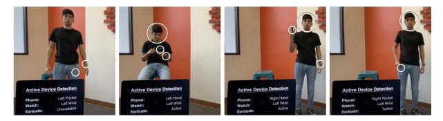
Figure 8.10: Active device tracking across different device combinations. Active devices are highlighted with a white circle for illustration and the foreground laptop shows the live tracking result.
