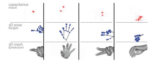
Figure 5.5: Top: Raw capacitive input images. Middle: Ground-truth hand poses for comparison. Bottom: Hand meshes rendered using skeletons that were estimated by TouchPose.
