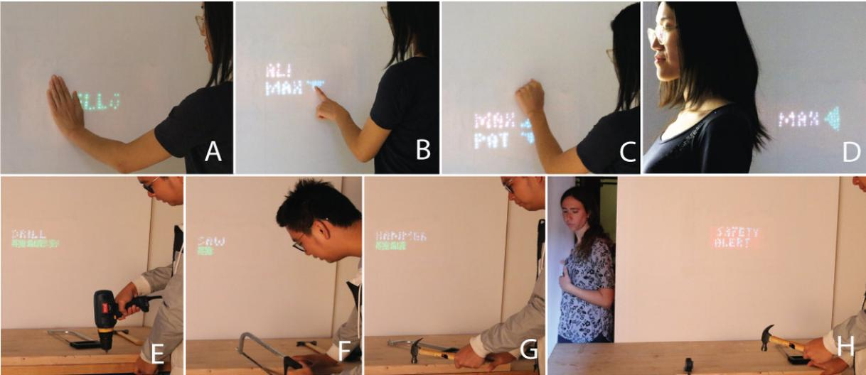
Figure 4.9: Applications of the Active Wall. An interactive contact directory application uses gesture input and visual feedback to guide users to where they need to go (A-D). A passive workshop activity recognition application senses what tools are being used (E-G) and warns users when another person enters the shop area to enhance workshop safety (H).
