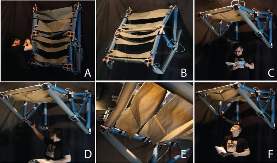
Figure 6.8: A walk-through of our interactive canopy with a user deploying it (a-b) and controlling the blinds via a swipe gesture (c-d) to receive more light (e-f).
