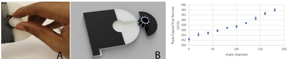
Figure 5.4: a) Shows the rotary encoders fabricated with FiberWire. The casing includes partially filled carbon fiber in semi-circle and the knob fully filled with carbon fiber b) Shows the assembly of the encoder c) Shows the characterization of capacitance vs angle of our rotary encoder design
