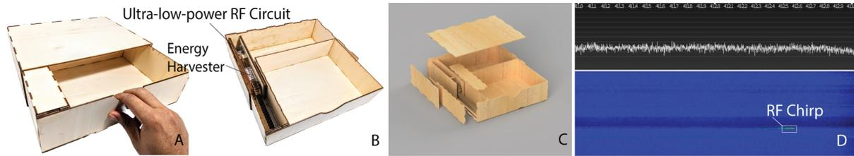
Figure 7.8: Shows interactive drawer, that harvests power from user pulling the drawer, to send a wireless interactive event
