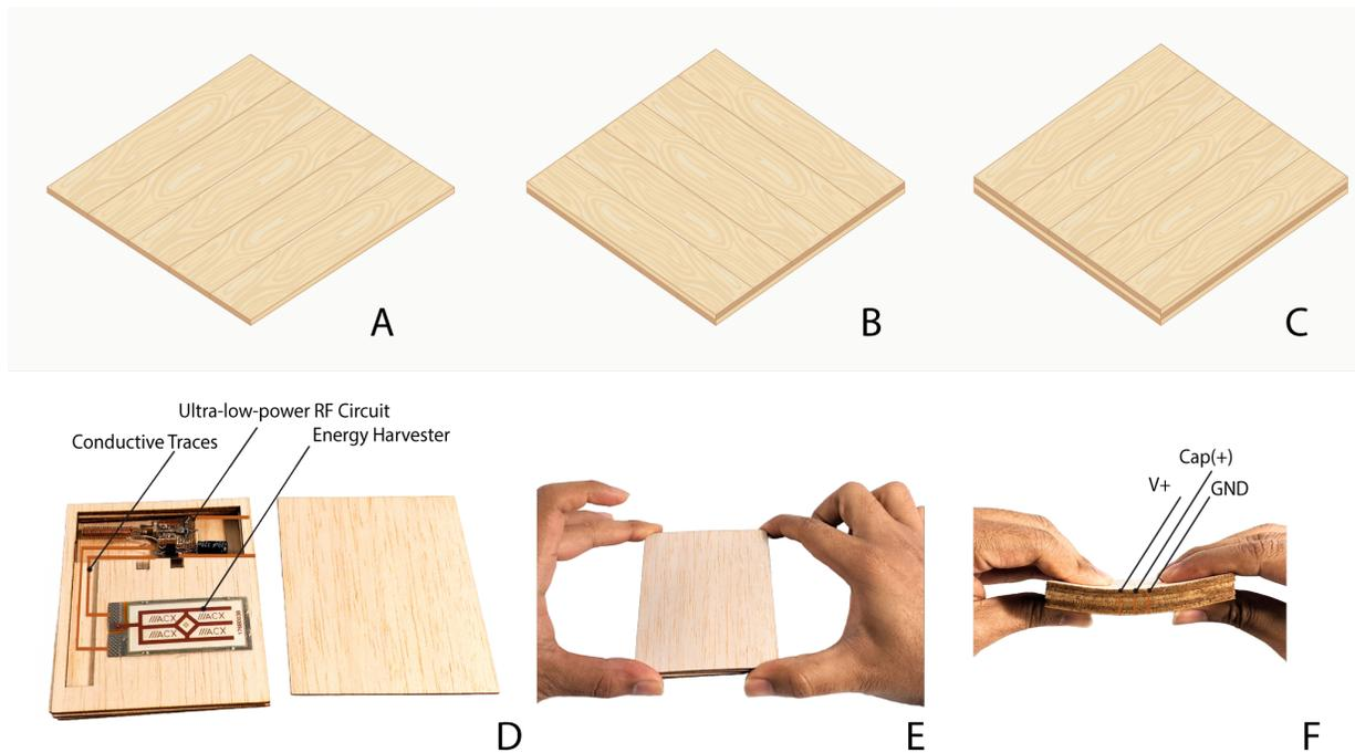
Figure 7.1: Shows the manufacturing process for computational wood, a six layer cross laminated ply of a relatively soft wood with embedded circuits and piezoelectric energy harvester
