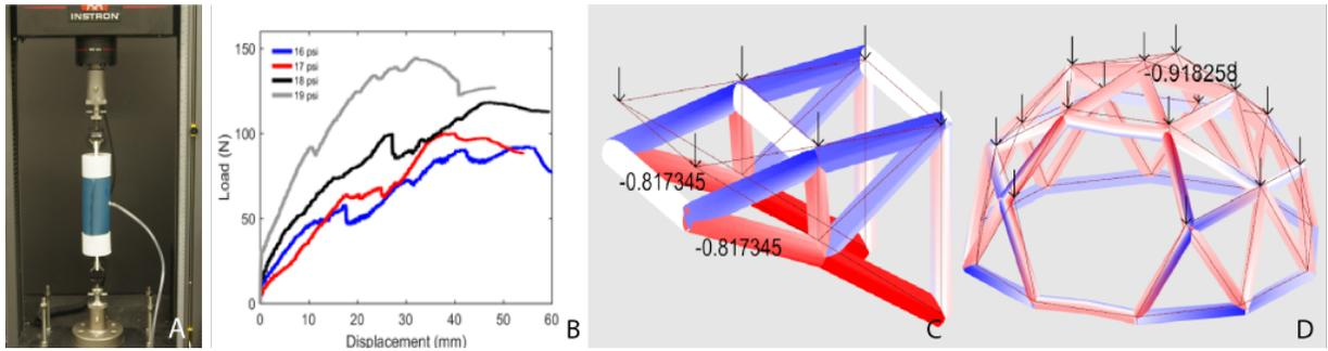
Figure 6.12: (a) Compression testing of an inflated truss member with an Instron 5969 testing machine. (b) Shows loading vs applied pressure behavior of truss elements under compressive load. (c) FEA analysis depicting the deflection of our truss frames from undeformed state. (d) Dome shows a deflection of 0.92cm from top and canopy shows a deflection of 0.81cm from tip of the roof.
