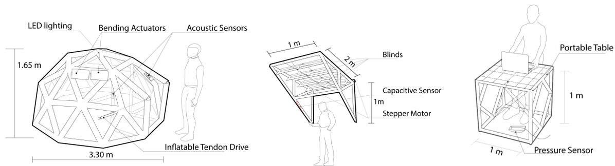
Figure 6.2: (a) An overview of an interactive geodesic dome with various actuators and sensors embedded as a part of the structure; showing the placement of contact microphones that are used to detect user gestures via swept frequency ultrasonic acoustic sensing; the various actuator mechanisms for door and windows (deployed) (b) Overview of interactive canopy structure with an embedded capacitive sensor for controlling blinds. (c) Portable table with embedded pressure sensing for deployment.
