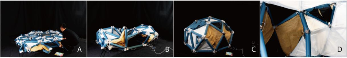
Figure 6.3: Shows a user connecting a pneumatic pipe (a) and the structure inflating itself (b) the structure is fully deployed (c) and the structure from inside (d).
