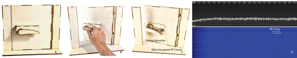
Figure 7.9: Shows interactions with a door handle, that harvests power from users mechanical action to send a wireless interactive event
