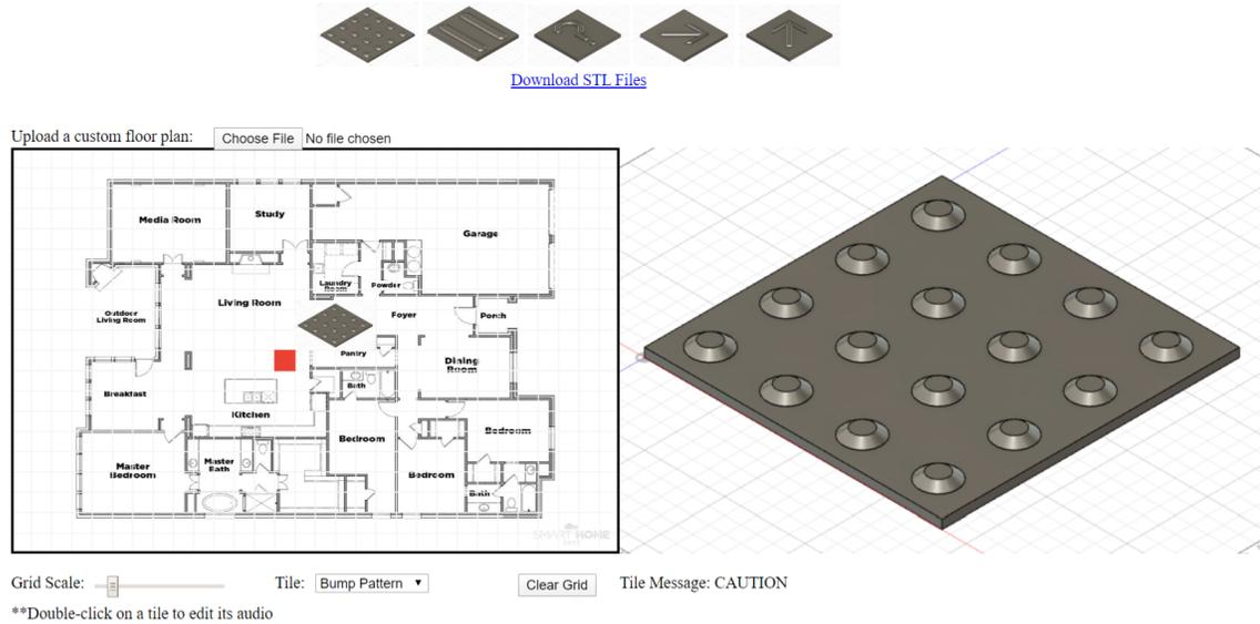
Figure 8.3: Shows a web application UI for custom planning of the tiles and recording audio prompts. This application is running on a web server and is sending audio prompts to users phone
