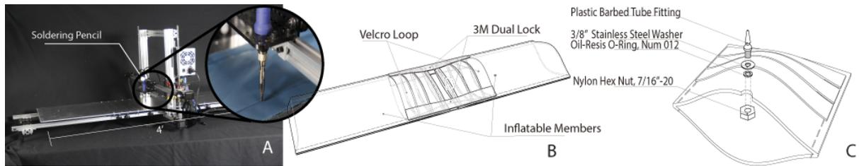
Figure 6.10: (a) Our customized heat sealing printer; Working condition of the soldering iron can be seen through inset. (b) Joints made between inflatable members with velcro hook and loop. (c) Exploded view of the composition of the inlet valve system.
