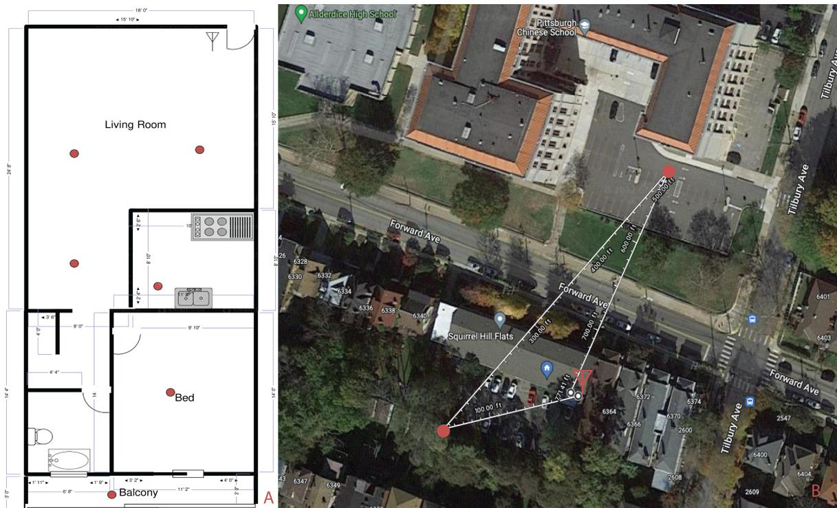
Figure 7.11: (a) Shows floor plan of house tested, transmission locations tested are represented by red dots (b) Shows testing range outside a residential building in two parking lots located 150 feet and 250 feet away
