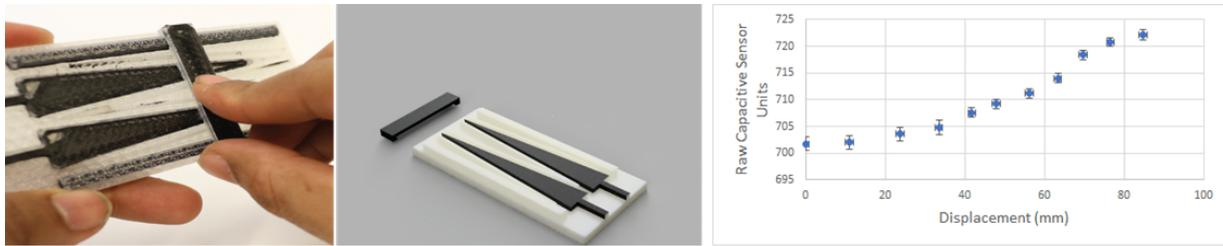
Figure 5.3: a) Shows the sliders fabricated with FiberWire. We used a triangular design varying the capacitor plate area b) Shows the assembly of the slider. Note that prints of all printed examples have been done using a white nylon base with black carbon fibers to make material placement apparent. c) Shows the characterization of capacitance vs displacement behavior of our slider across the device
