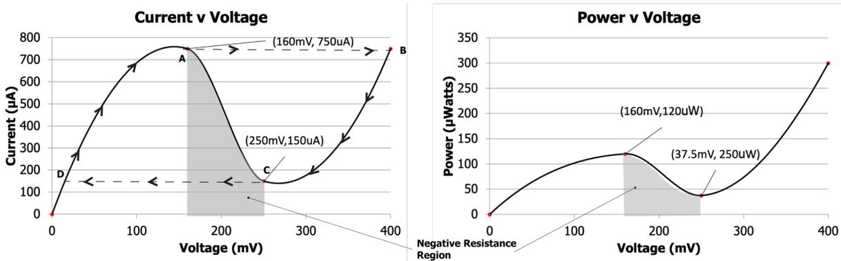
Figure 7.4: Shows current vs voltage and the power vs voltage graph for biasing the tunnel diode in the region of interest
