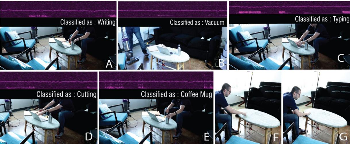
Figure 4.12: Applications of the active table including activity recognition of interactions on and around the table (A-E) and a gesture based music player that uses tap, swipe, and knock. as input control for a music player.
