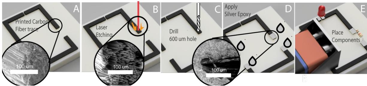
Figure 5.1: FiberWire Fabrication workflow: (a) 3D printing of carbon-fiber trace circuit, inset shows SEM image of the carbon-fibers bonded with epoxy in the resin matrix (b) Laser etching of epoxy to expose raw carbon fibers, inset shows results of laser etching (c) Drilling micro holes for interfacing with electronic component pins (d) Deposition of silver epoxy on exposed carbon fiber, inset shows carbon fibers are coated with conductive silver and (e) Placement of the components
