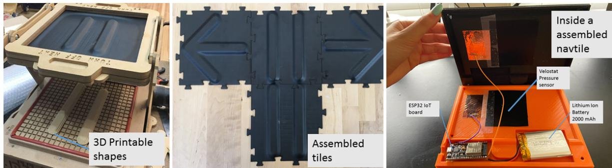
Figure 8.4: (A) Shows 3D printable textures and a thermoformer for making a texture, (B) Shows guidance surfaces inter-locked with each other (C) Underlying electronics, a sensor to make the tiles multi-modal.
