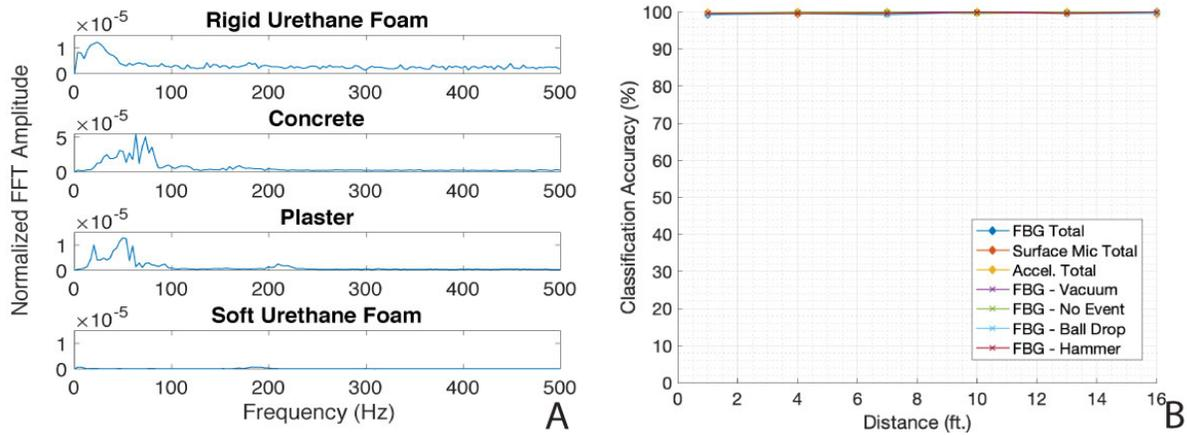
Figure 4.5: (A) Frequency responses for different materials subjected to an impulse hammer excitation. Note the changes in frequency content for each material. (B) Shows Combined classification accuracy of our system with varying distance. We observe that with distances of up to 16 ft, there is not an appreciable decrease in performance of our system.
