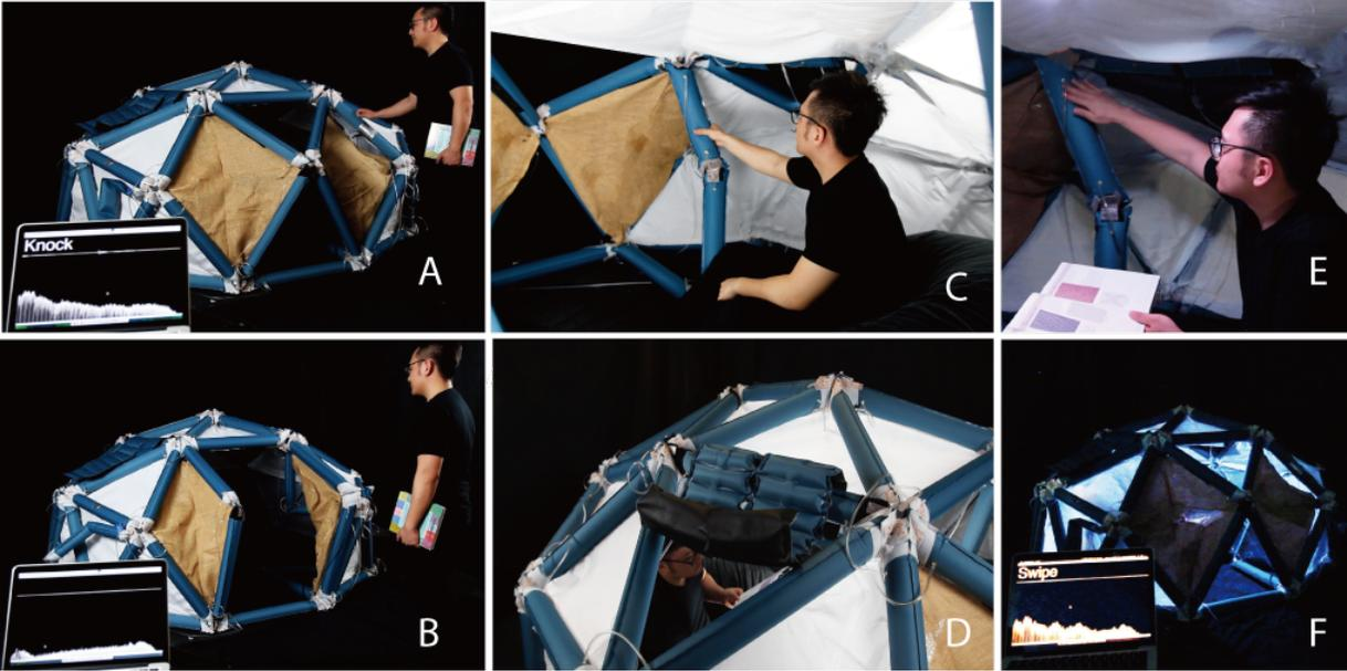
Figure 6.4: (a) shows a user performing a knock gesture and our system recognizing user input; (b) shows the door opening for the user to enter.(c) shows a user performing a squeeze gesture; (d) shows the windows of the dome rolling up in response.(e) shows a user performing a swipe gesture; (f) shows the lighting switched on inside the dome.
