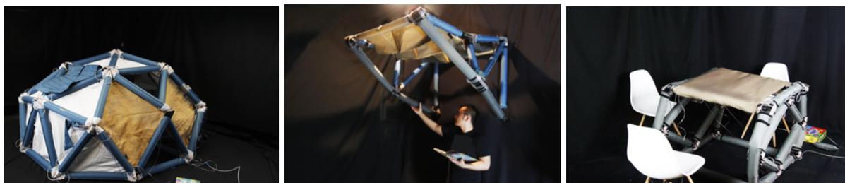
Figure 3.2: (a) A geodesic dome that deploys itself upon inflation and has embedded actuation and acoustic sensing to open its doors and raise its windows; (b) a canopy with a controllable venetian blind via capacitive sensing; (c) a portable table inflated on-demand via a pressure sensitive control. All of these structures have embedded actuation and sensing that support a range of interactions (e.g., a user performs a knock gesture on the dome’s door and the door swings open).
