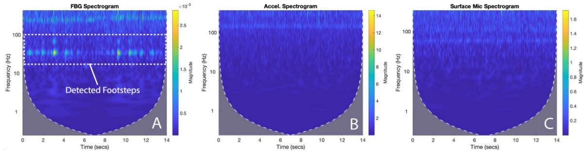
Figure 4.6: Spectrogram showing the footstep detection at a distance of 16 feet for three sensors – FBG (A), accelerometer (B) and surface microphone (C). Note that the FBG can clearly detect many of the footsteps, while there is no visible response from the other two sensors.
