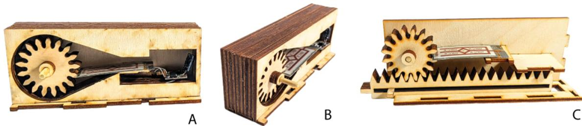
Figure 7.2: Shows various energy harvesting mechanisms that are embedded within plies of cross laminated wood
