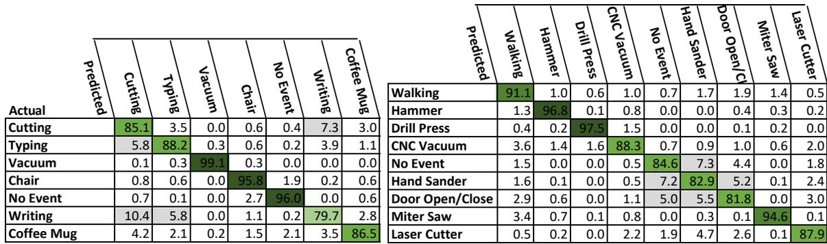
Figure 4.11: Confusion matrices for various events on two interactive structures. (A) shows performance of embedded coffee table unit in identifying various activities. (B) shows performance of the active wall in identifying various shop activities.
