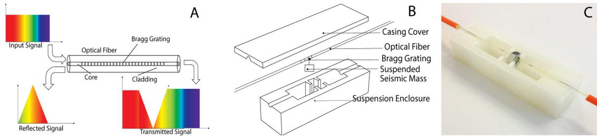
Figure 4.1: Fiber-Bragg Grating Optical Sensing and hardware. The Fiber-Bragg Grating Optical Sensor uses Bragg gratings on an optical fiber to reflect different amounts of light based on an input signal (A). The input signal is captured on a vibration transducer that houses the optical fiber (B and C).
