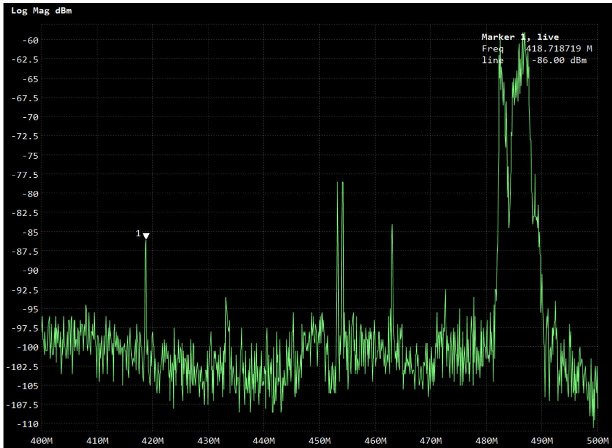
Figure 7.6: Power spectrum of our oscillator peak at 3m distance. We generate a signal in the 418 MHz band, at a peak biasing power of 120  $\mu$ W.
