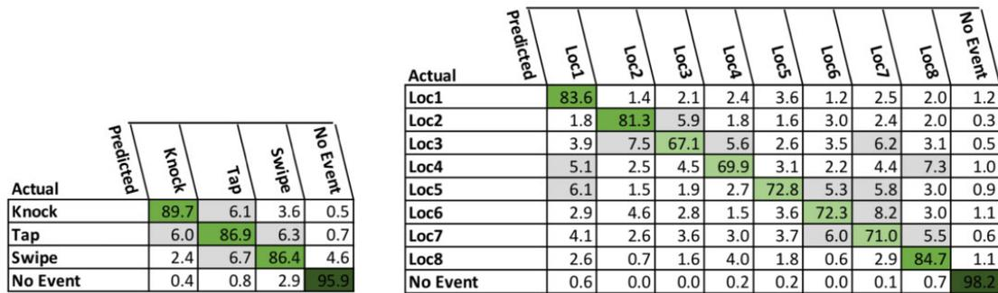
Figure 4.10: Active wall classification accuracy for gestures in user studies with 8 participants. The left confusion matrix shows performance of the prototype in identifying common wall gestures (knock, tap, and swipe) across 8 participants. The right confusion matrix shows performance of the active wall in identifying tap locations across 8 participants.
