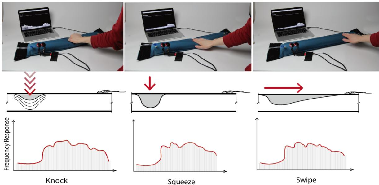
Figure 6.5: Using swept frequency ultrasonic acoustic sensing, we are able to distinctly identify a number of gestures when performed on our inflated truss members. Note that the frequency responses above refer to the ultrasonic region (displayed in the far-right of the laptop screen).
