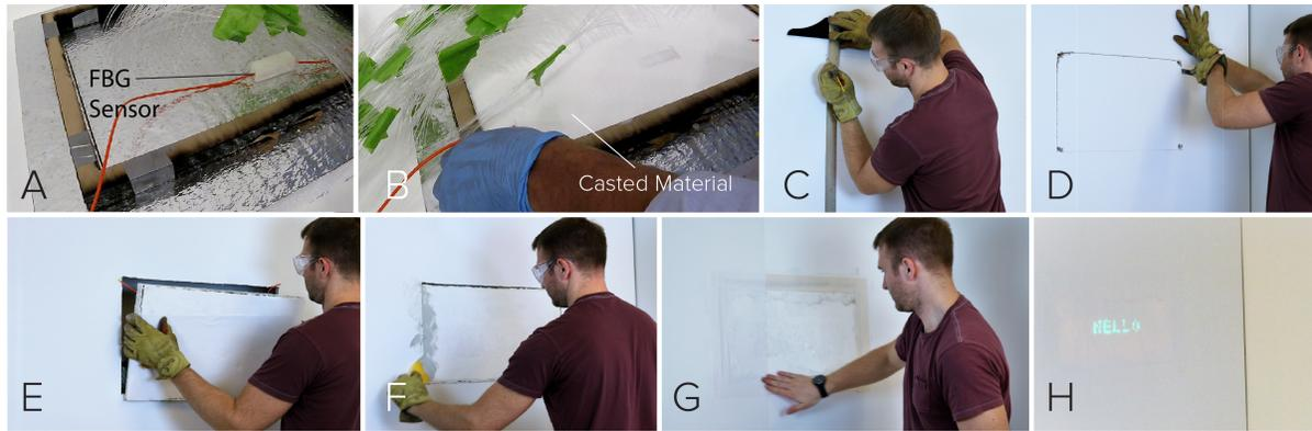
Figure 4.7: Fabrication Process for Active Wall. A FBG sensor is placed into a rectangular mold containing an injected fiber optic display (A). Material is cast into the mold (B). A region of an existing dry wall is removed and replaced with the cast structure (C-G). Finally, the display output of the optical fibers is tested and reveals the message “Hello” on the wall (H).
