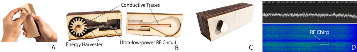
Figure 7.7: Shows handheld interactive input control device made from wood, rotating the knob by 180 degrees, sends a wireless event
