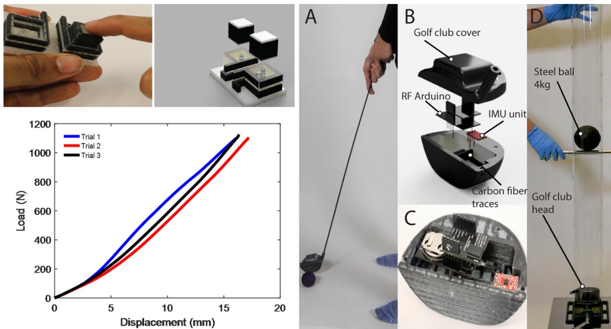
Figure 5.6: a) Shows the golf club with a user b) Shows the exploded view of golf club with RFduino and accelerometer c) Shows the top view of the fabricated sample d) Shows the drop ball impact test of the golf club head. e) Bike Handle Bar Strength Testing f) Shows the fabricated tactile buttons with two fiber traces embedded with a nylon layer in the middle. g) Shows the caps that go with the buttons which are also fabricated with carbon fiber
