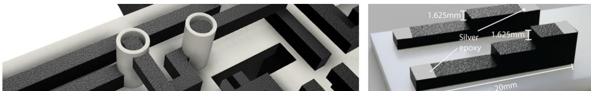
Figure 5.2: a) Shows cylindrical via printed between traces layers b) Resistance characterization test between layers
