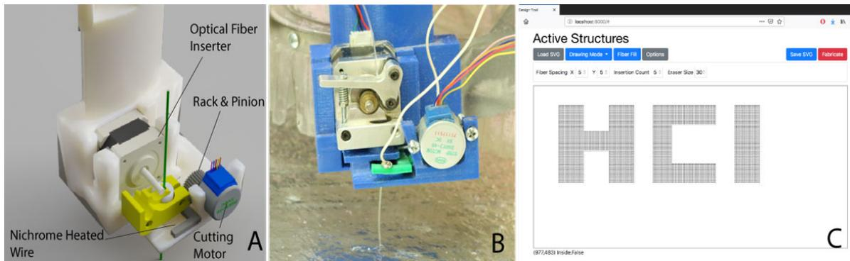
Figure 4.4: Optical Fiber Inserter and Cutter Assembly (A), insertion process (B) and design software (C).
