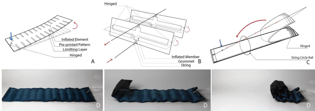
Figure 6.7: (a) rolling bend actuator implementations (b) twisted tendon drive, and (c) Our inflated tendon drive. (d) Our rolling bend actuator shown in bottom half rolling upon inflation
