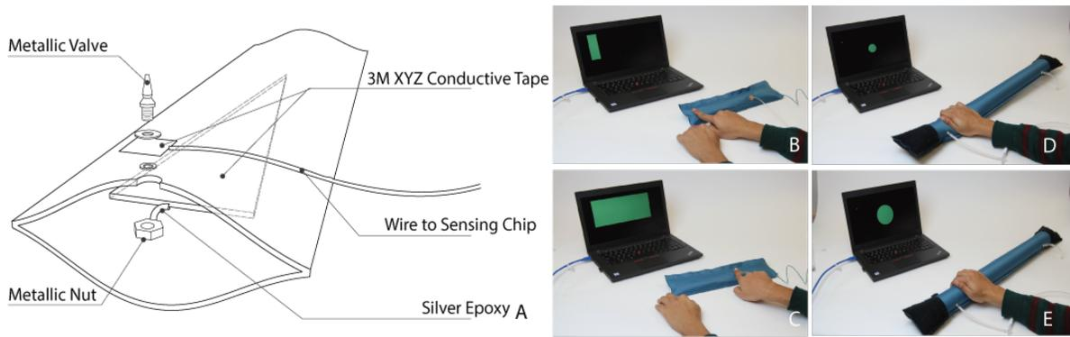
Figure 6.6: (a) Technical drawing of our capacitive slider implementation embedded into the inflatable member; (b) shows a user beginning their finger along the member; (c) shows the visualized output on a laptop display (d & e) Our pressure sensing implementation: as a user applies force to the inflated member and the pressure is visualized on the laptop display.
