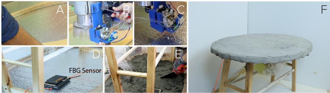
Figure 4.3: Fabrication Process for Active Cement Table including milling a mold using a CNC mill (A); attaching the fiber insertion hardware to the mill (B); inserting the optical fibers (C); placing the FBG Sensor (D) into the mold; casting cement into the mold (E); and the finished table (F).
