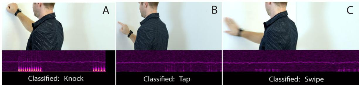
Figure 4.8: A variety of surface gestures such as a knock (A), tap (B) and swipe (C) can be reliably detected in discrete locations as seen in their respective spectrograms.
