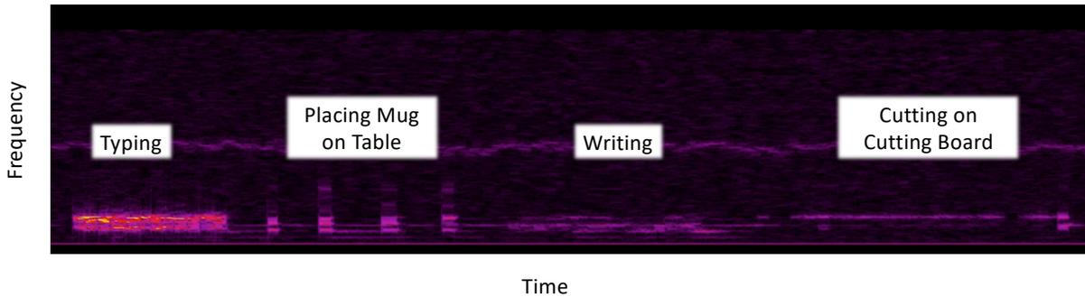
Figure 4.2: Spectrogram showing the vibration response variation for different activities on an instrumented table. Color variations represent changes in intensity/magnitude.
