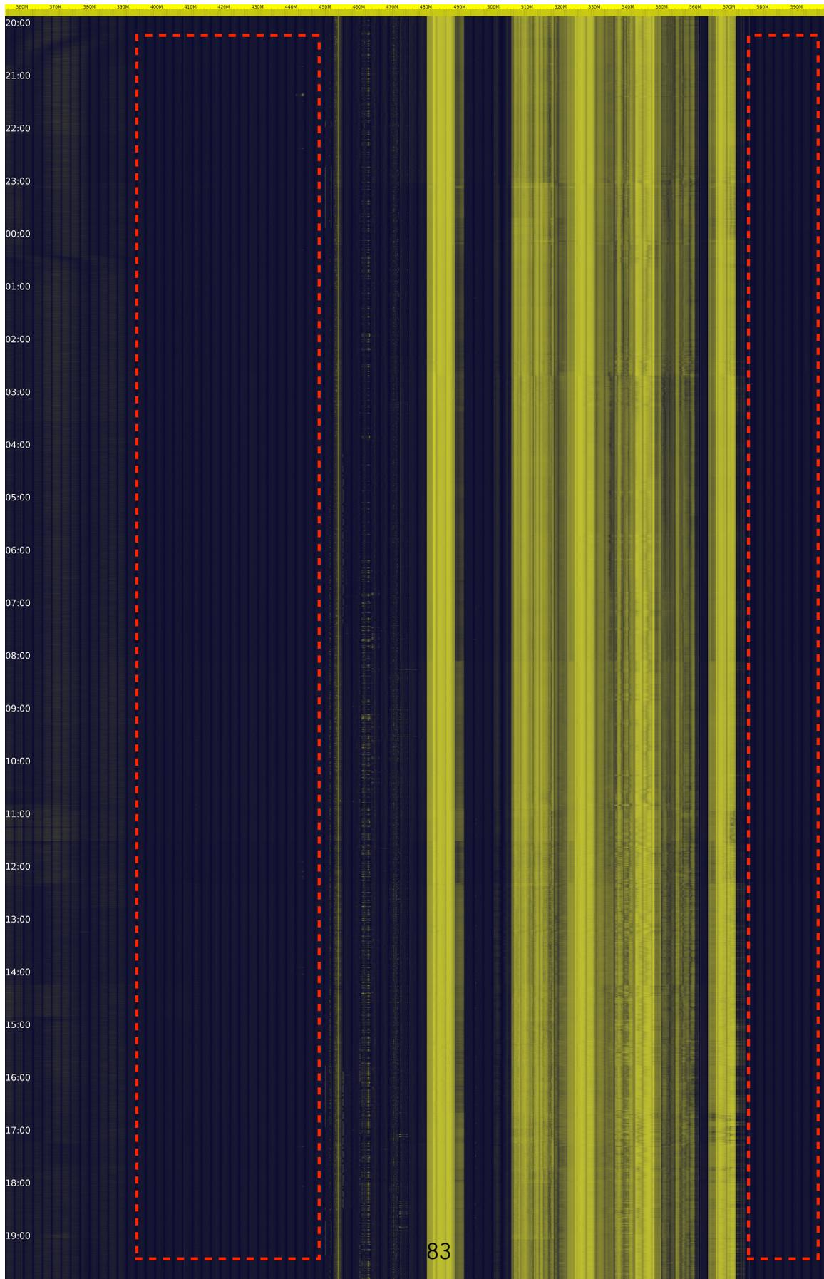
Figure 7.5: A 24-hour spectrum data for 350MHz-600MHz. The dotted red line indicates quite parts of the spectrum that can be used for sending broadcasts
