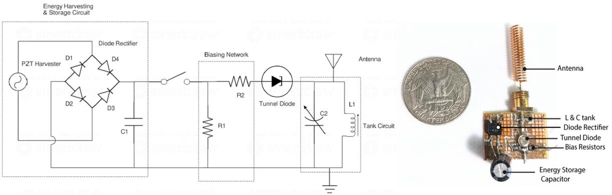
Figure 7.3: Shows energy harvesting, storage and ultra-low-power RF circuit constructed with tunnel diode
