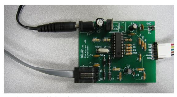
Figure 4-2. Circuit for the Telephone Tracker sensor that plugs into the phone line and monitors when the phone is on/off the hook and which numbers are dialed.
