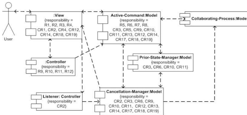
**Figure 4-2. UML-style component diagram of MVC revised to include the responsibilities necessary to provide the ability to cancel a long running command. New cancellation responsibilities are numbered CR1, CR2, etc., are assigned to both old and new components, and refer to prose descriptions of the responsibilities in the Cancellation USAP.**
