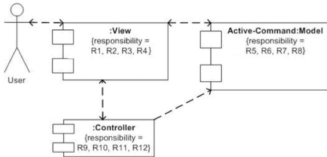
**Figure 4-1. UML-style component diagram of the MVC reference architecture before considering the ability to cancel a long running command. Original responsibilities of MVC are numbered R1, R2, etc. and refer to prose descriptions of the responsibilities accompanyi**
