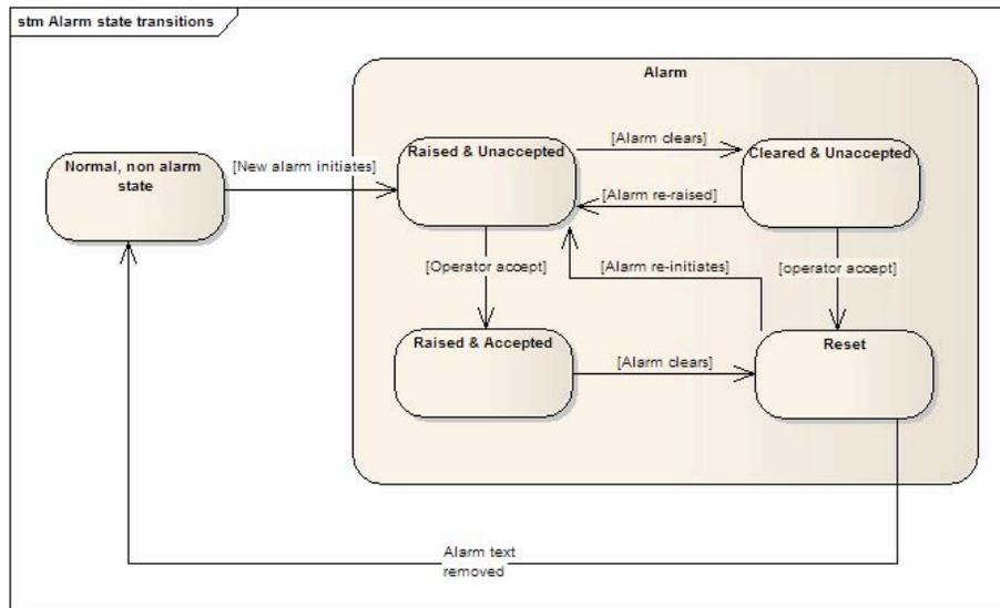
Figure 2. EEMUA's definitions of alarm state transitions.
