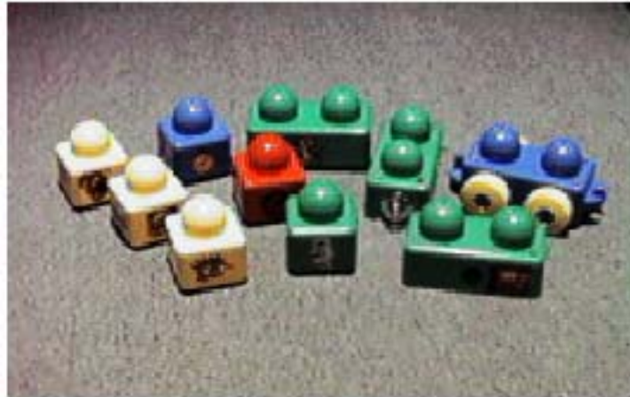
Figure 11.10: Electronic Blocks: the three sensing blocks are pictured on the left, the logic blocks in the middle, and the action blocks on the right
