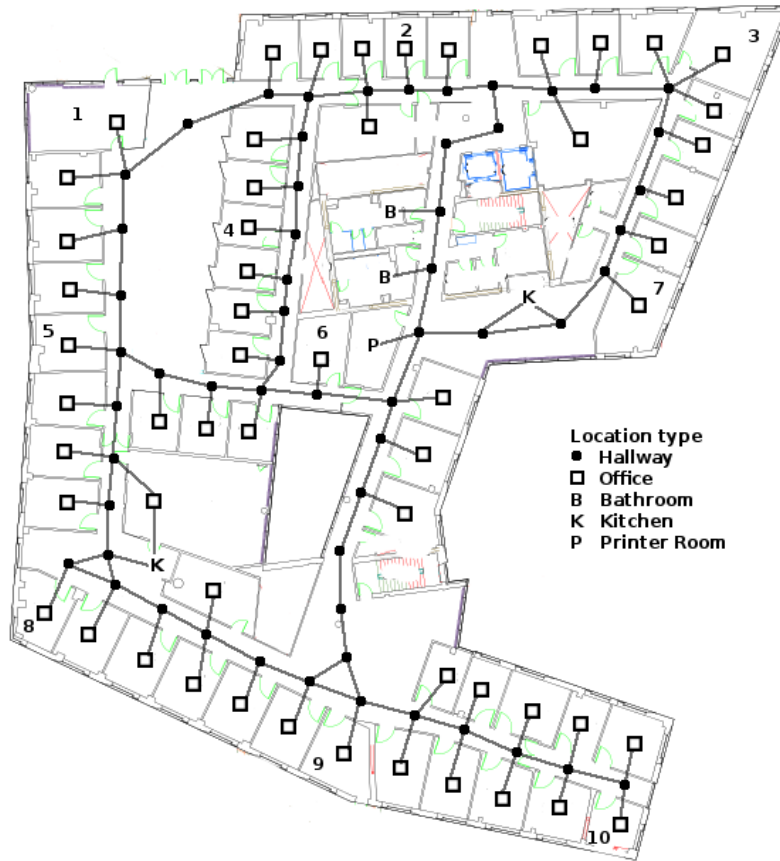
Figure 8.5: Floor plan used in our service robot experiments. The embedded graph represents the map given to the planners. The initial location for the experiments are represented by the numbers 1, ..., 10.
