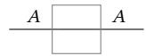
Figure 9.5: A well-typed empty chain that uses service A to offer service A
