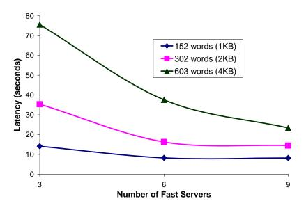
The Figure shows the effect of data decomposition for three different inputs. The x-axis is the number of servers used and the y-axis is the overall application latency. The servers are used in groups of 3 because panlite's tactic has 3 parallel stages.
