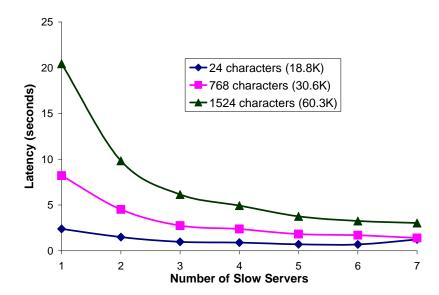
The Figure shows the effect of data decomposition for three different inputs. The x-axis is the number of servers used and the y-axis is the overall application latency.
