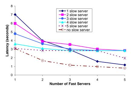
The Figure shows the effect of data decomposition in a heterogeneous environment. The x-axis is the number of fast servers used and the y-axis is the overall application latency. Each line represents the number of slow servers used.
