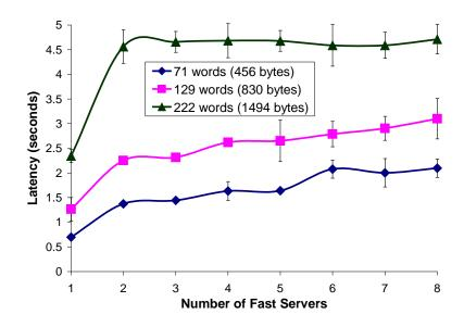
The Figure shows the effect of an inefficient join function for three different inputs. The x-axis is the number of servers used and the y-axis is the overall application latency.
