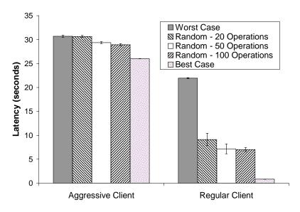
The Figure shows the effect of random server selection for two clients (each client selecting 2 servers from a set of 8). The worst case occurs when both clients use the same servers. The next three bars show the effect of random server selection for different numbers of concurrent operations for the regular client. The final bar shows the best case performance where each client uses separate servers.
