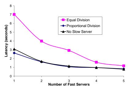
The Figure shows the effect of proportional data decomposition in a heterogeneous environment. The x-axis is the number of fast servers used and the y-axis is the overall application latency. The base case is the "No Slow Server" case. The other two lines show the effects of using a single slow server with proportional and equal data division.
