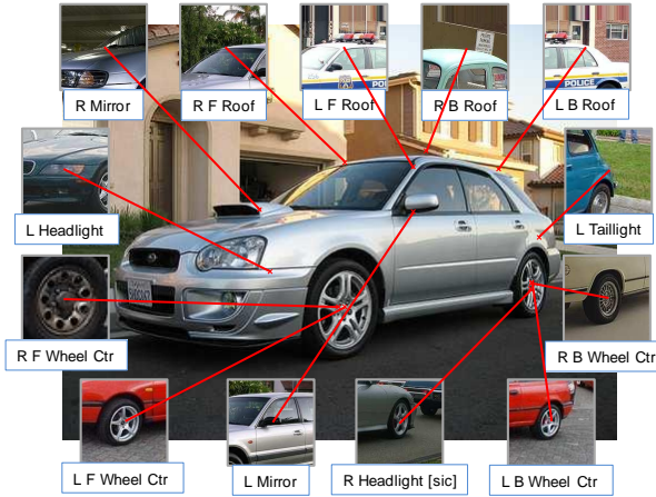
Figure 5.10: An example of keypoint transfer. For each predicted keypoint, we show a patch from the image where that keypoint was transferred from. These correspondences are discovered without any supervision. Note that multiple different labels are predicted for the wheel centers. This happens because our algorithm finds all wheels somewhat visually similar, and proposes as many correspondences as possible.
