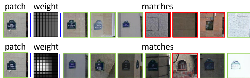
Figure 3.5: Top: using the naïve distance metric for this patch retrieves some good matches and some poor matches, because the patch contains both a street sign and a vertical bar on the right. Bottom: our algorithm reweights the dimensions of our patch descriptor to separate Paris from non-Paris. The algorithm learns that focusing on the street sign achieves maximum separation from the non-Paris walls.
