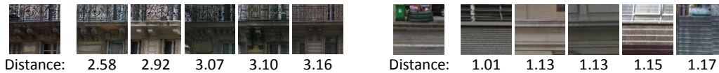
Figure 4.1: The distribution of patches in HOG feature space is very non-uniform and absolute distances cannot be trusted. We show two patches with their 5 nearest-neighbors from the Paris Street View dataset [43]; beneath each nearest neighbor is its distance from query. Although the nearest neighbors on the left are visually much better, their distances are more than twice those on the right, meaning that the actual densities of the two regions will differ by a factor of more than 2^d , where d is the intrinsic dimensionality of patch feature space. Since this is a 2112-dimensional feature space, we estimate d to be on the order of hundreds.
