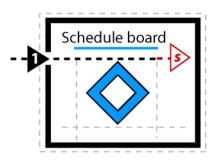
Figure 4-12. Schedule board and control desk are in a core area for authorized workers only; non-authorized persons circulate around the perimeter.
