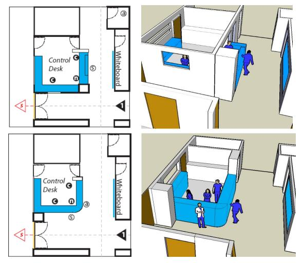
Figure 4-6. (Top) Large Surgical Suite as it was during the field study. (Bottom) Concept sketch with open control desk and more space to accommodate people around both sides of the control desk undisturbed by indoor traffic.
