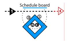
Figure 4-10. Information access areas around the schedule board and control desk allow key decision makers to congregate. The *a* represents the charge anesthesiologist, *n* the charge nurse, *c* the clerk, and *s* the surgeon. The dotted semicircle indicates an area around the schedule board where decision makers can congregate.
