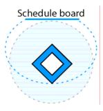
Figure 4-7. Schedule board and control desk are mutually visible and close enough to be mutually accessible. The donut represents the control desk and the dotted lines are where the schedule board and control desk are accessible.
