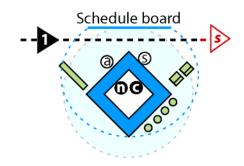
Figure 4-11. Benches, stools, or chairs (rectangles, circles) around the control desk (large square), with a view onto the schedule board encourage multiple activities. The a represents the charge anesthesiologist, n the charge nurse, c the clerk, and s the surgeon.
