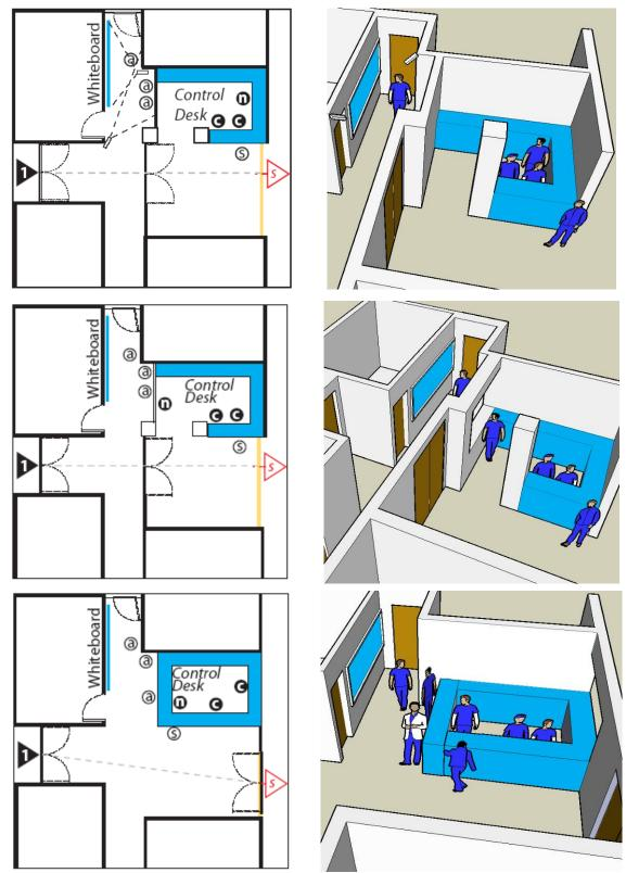
Figure 4-5. (Top) Video and audio links connect the whiteboard area and the control desk. (Middle) A glass window and audio link connect the whiteboard area and the control desk. (Bottom) New control desk adjacent to the whiteboard and lounge.
