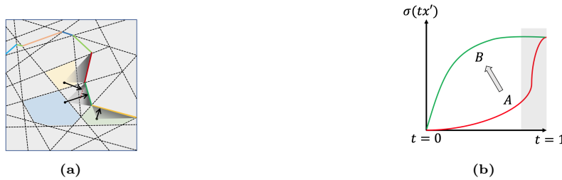
Figure 4.2: (a) A geometric view of the input space in a ReLU network. Dashed lines correspond to activation constraints while the colorful solid lines are piece-wise linear decision boundaries. Taking gradient of the model's output with respect to the input returns a vector that is orthogonal to a nearby boundary (points in the blue and green regions) or an extension of a nearby boundary (the point in the yellow region). (b) Curves of the model's sigmoid output \sigma(tx') (y-axis) against interpolation parameter t (x-axis).
