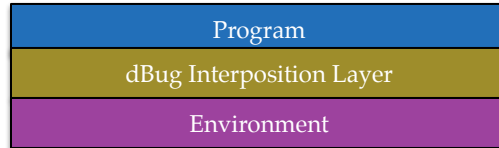
Figure 3.7: Monitoring Program Behavior with dBug Interposition Layer
