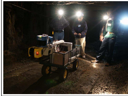
Figure 2: Mine mapping cart with four laser range finders, for our new 4x2-D volumetric mapping approach.
