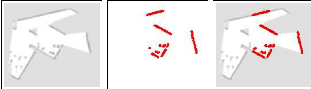
Figure 3: Two-dimensional scan alignment. Map created out of the most recent scans (left image), range scan measurement (center image), and resulting alignment (right image).
