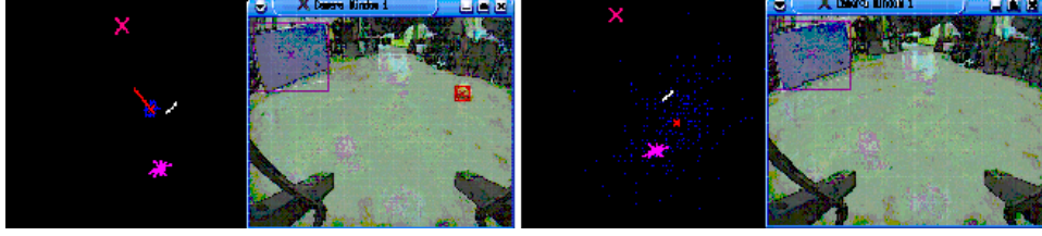
Figure 4: In both figures, the red and pink cross represent the two goals, and each blue dot represents the one of the particle estimation of the ball position. In the left figure, the ball is visible to the robot. In the right figure, the ball is out of sight and the particles are scattered
