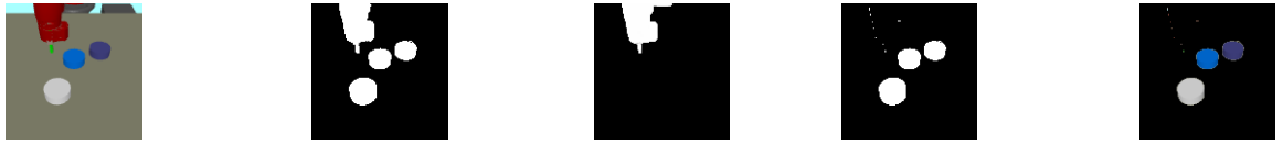
(a) original image (b) foreground mask (c) robot mask (d) object mask (e) segmented objects
