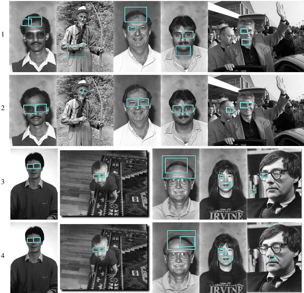
Figure 57: These are examples of detections generated by the detector on the test set before and after the use of weakly labeled data. The two detections with the highest confidence values are plotted with a green box scaled according to the detection size. Rows 1 and 3 contains example detections with the fully labeled data subset only. Rows 2 and 4 contain example detections with the addition of weakly labeled. The examples in row 2 show improvements over those in row 1 with the use of weakly labeled data. The examples in row 4 show no improvement or some degradation with the use of weakly labeled data.
